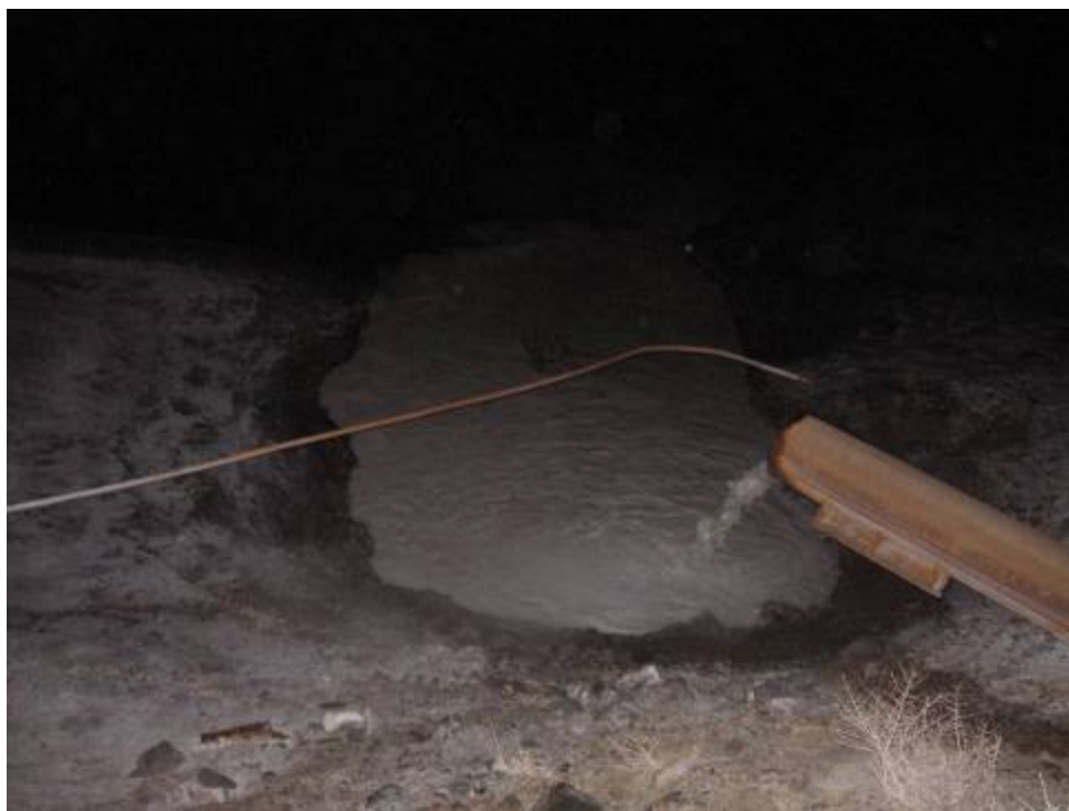
Figure 19. Picture of the produced fluid from 32A-20 to the adjacent pit about 3 hours after the well was opened. Note the milky-white color of the produced fluid indicating the calcium-NTA complex.
