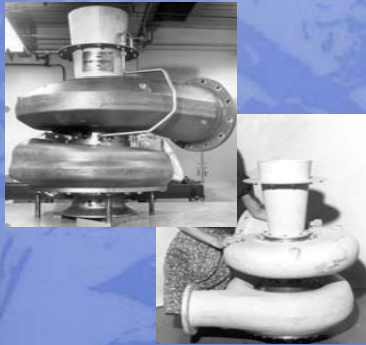
2 Bootstrap Turbochargers (Full and Partial Flow Sizes) TEPCO 5MW Phosphoric Acid Fuel Cell Power Plant 1981
