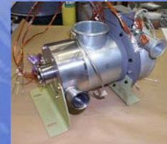
Demonstration of Motor Driven Turbocharger w/Mixed Flow Compressor and Variable Nozzle Turbine DoE 50kW PEM Fuel Cell System for Light Duty Vehicle 2001
