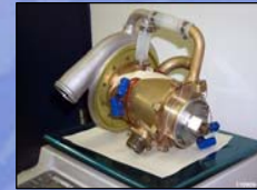
Motor Driven Turbocharger PEM Fuel Cell System for Unmanned Aerial Vehicle 2003
