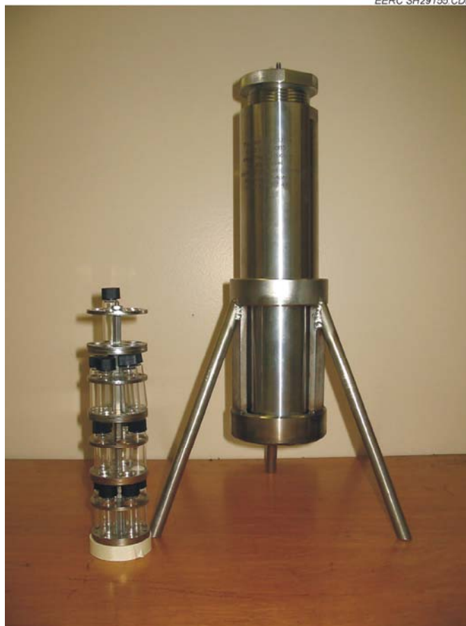
Figure 3. Apparatus for long-term exposure of twenty samples to carbon dioxide. The rack of sample vials on the left is placed into the pressure vessel, which is then attached to the carbon dioxide supply and placed in an oven.
