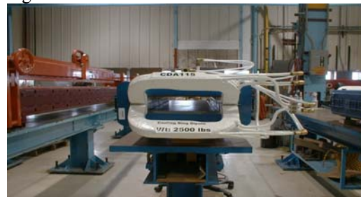
Fig. 8 CDA dipole for the HTS and LTS conductor tests CDA magnet at 0.7 T with repetition rates up to 5 Hz will exceed even multiple times the DSFMR magnet design parameters. The CDA magnet has a very large gap (82.5 mm height x 305 mm width) facilitating installation of the test conductors, and their removal from the magnet for e.g. the di/dt induced power loss measurements. For these measurements the power supply will be powered to
