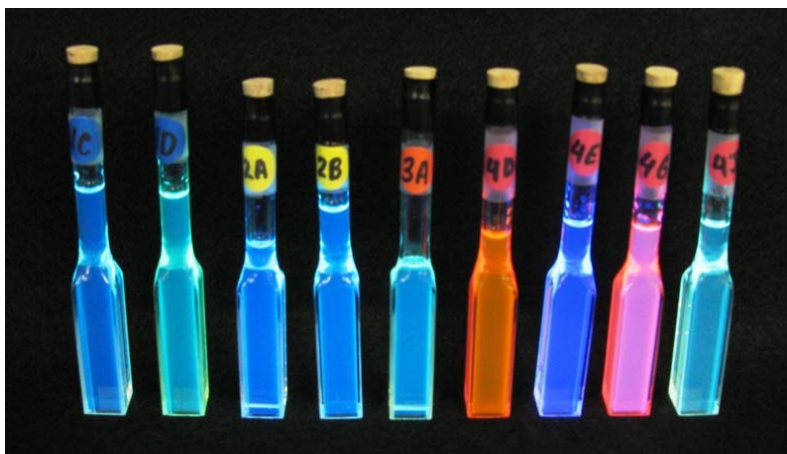
Figure 41. Several liquid scintillator samples in quartz cuvettes, excited under a black light. Left to right: Sample 1C (PXE + PPO + DSB1); Sample 1D (PXE + PPO + DSB2); Sample 2A (Pseudocumene + PPO + DSF1); Sample 2B (PXE + PPO + DSF1); Sample 3A (Pseudocumene + PPO + DSF2); Sample 4D (PXE + AH238B); Sample 4E (PXE + BBOT); Sample 4G (PXE + BBOT + AH238B); Sample 4J (PXE + b-PBD + BBQ).
