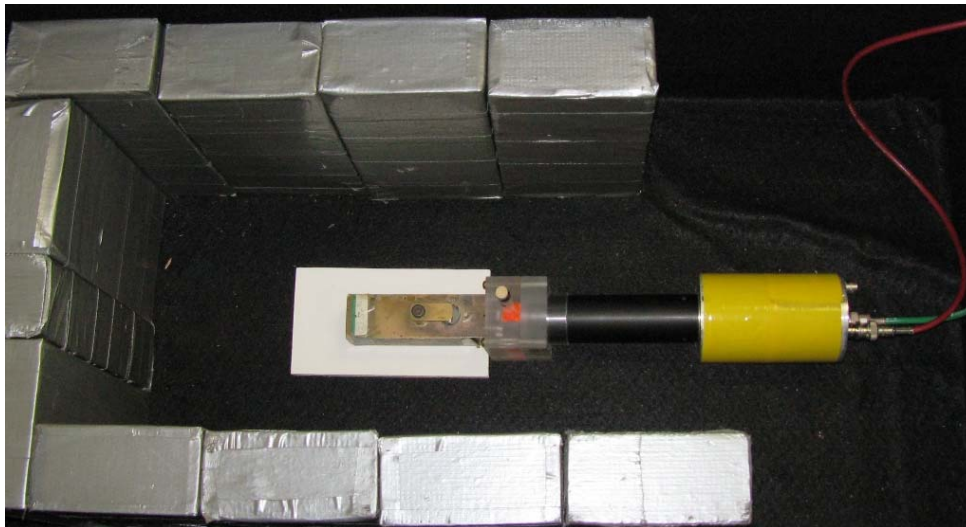
Figure 42. View of the geometric arrangement of the bulk tests of scintillating liquids and solids for efficiency. Excitation of the system was via electrons from a ^{90}\text{Sr} source. The photosensor was an R1104 multialkali PMT and readout was via a LeCroy QVT into a computer.
