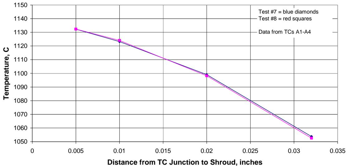
**Figure 45 Indicated Shroud Temperature versus Junction Displacement, Tests 7 & 8, TCs A1-A4**
