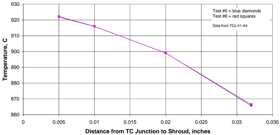
**Figure 44 Indicated Shroud Temperature versus Junction Displacement, Tests 5 & 6, TCs A1-A4**
