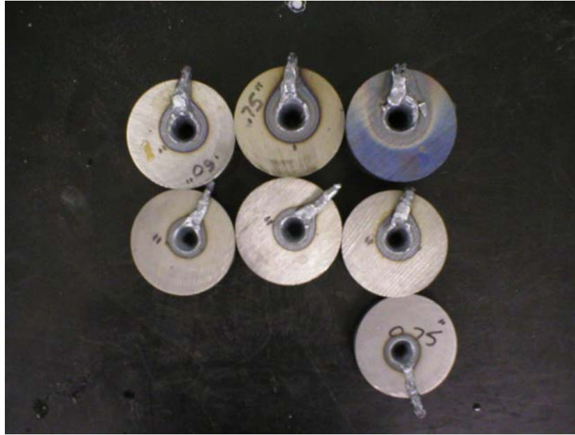
Figure 54. Steel sample at different thicknesses after lasing The second methods was by moving the robot in a circular motion to cut a circle as shown in figure 55.
