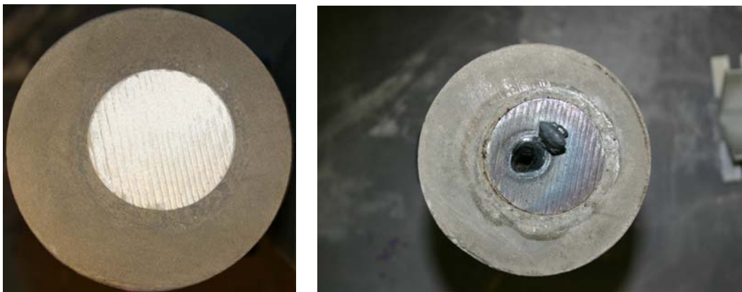
Figure 28. Pre- and post-laser images of 10.16 cm (4.0 in) diameter by 15.24 cm (6.0 in) length limestone core inset with 5.08 cm (2.0 in) diameter by 1.27 cm (0.5 in) thick steel plate.
