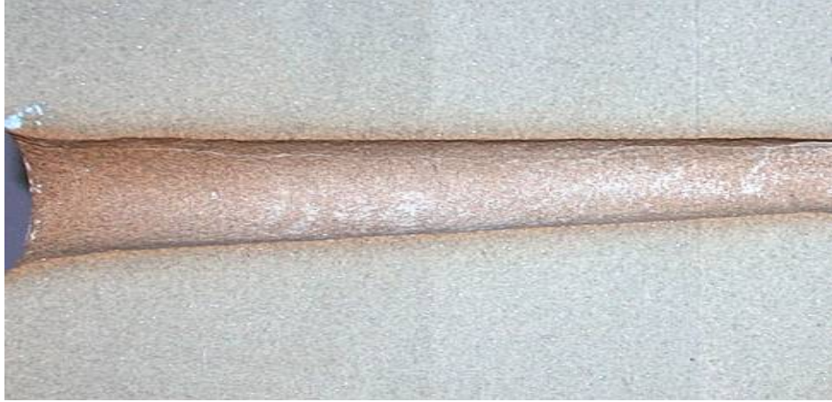
Figure 118. Deep hole in sandstone by spallation, the hole was clean without melt or debris and SE of 4 kJ/cc, Diameter of 1 inch with 12 inches long
