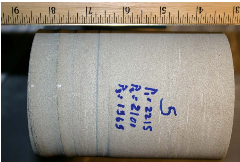
Figure 106. Fracture developed in limestone sample when stress was applied
