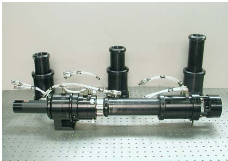
Figure 84. Collimator for HPFL collimates beam from 0.25" to 1"
