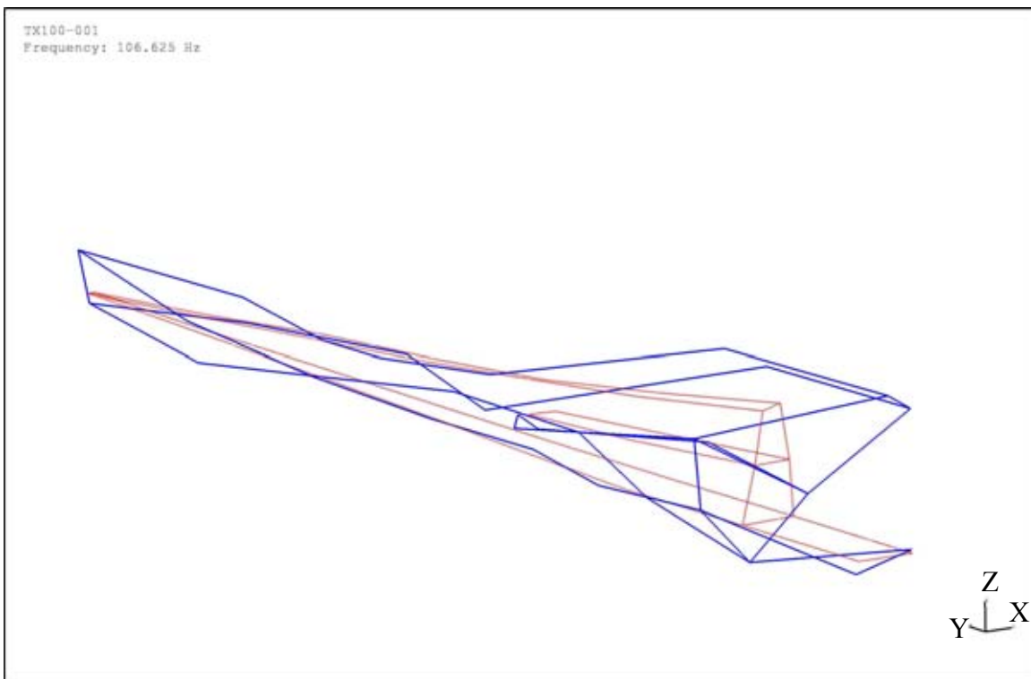
Figure A-15. Third Torsional Mode ( f = 107.13 Hz, \zeta = 0.73 %) Blade Serial #TX-100-001
