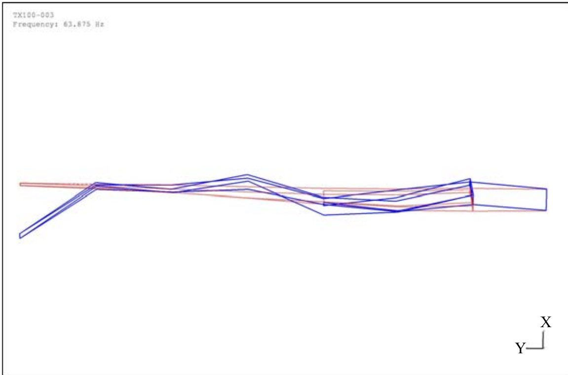
Figure B-8. Fifth Flapwise Mode ( f = 64.20 Hz, \zeta = 0.31\% ) Blade Serial #TX-100-003
