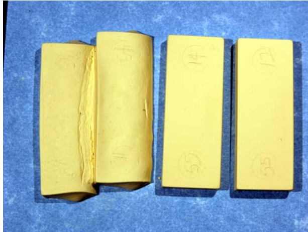
Figure 13. "Slumping" in 5% Surfactant Parts
