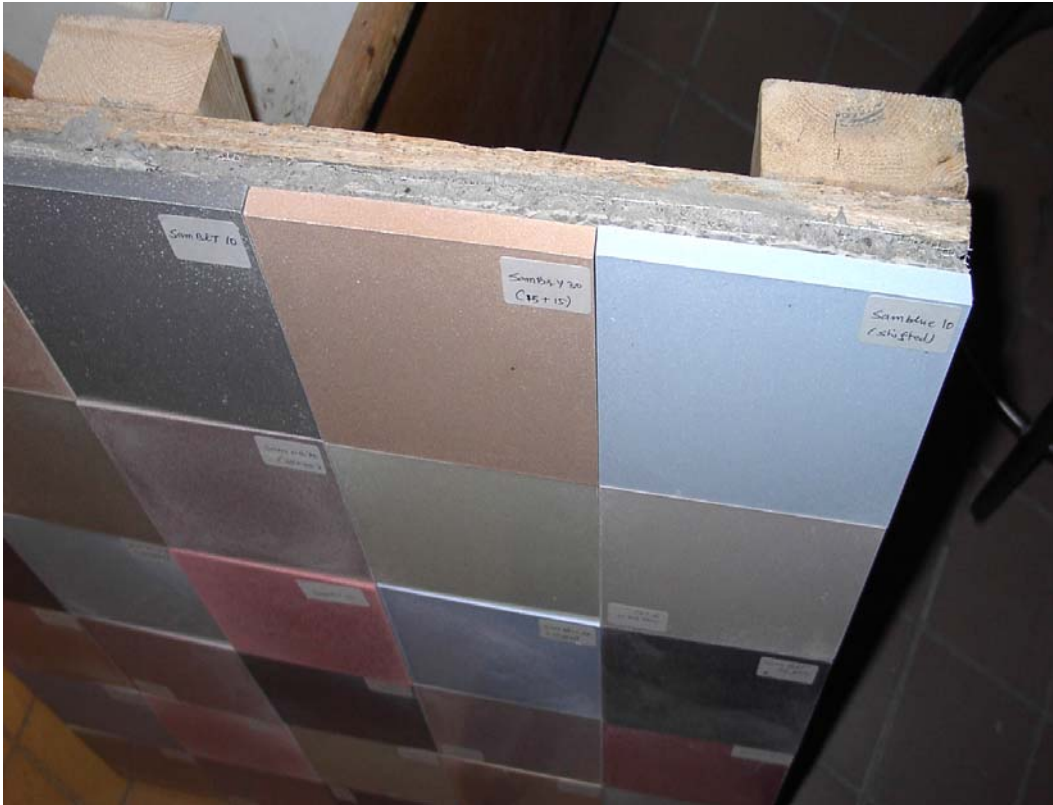
Figure 26. Excellent bonding was observed between tiles, fabricated from sulfate-rich scrubber sludge, and commercial Durock board as can be seen here.
