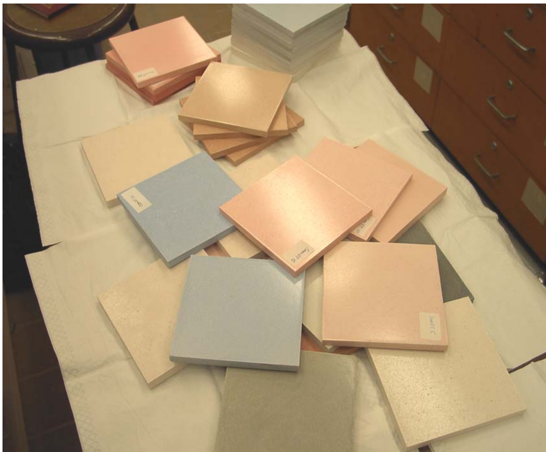
Figure 21. Decorative tiles made from sulfate-rich scrubber sludge and waste or broken tiles.
