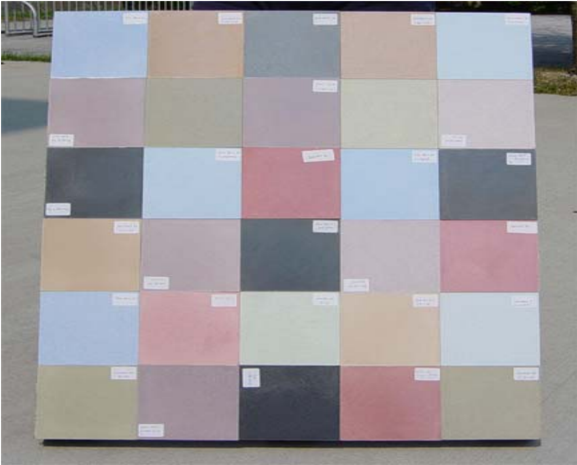
Figure 24. This figure shows thirty decorative tiles, which were mounted on a 3 feet by 2.5 feet Durock board.
