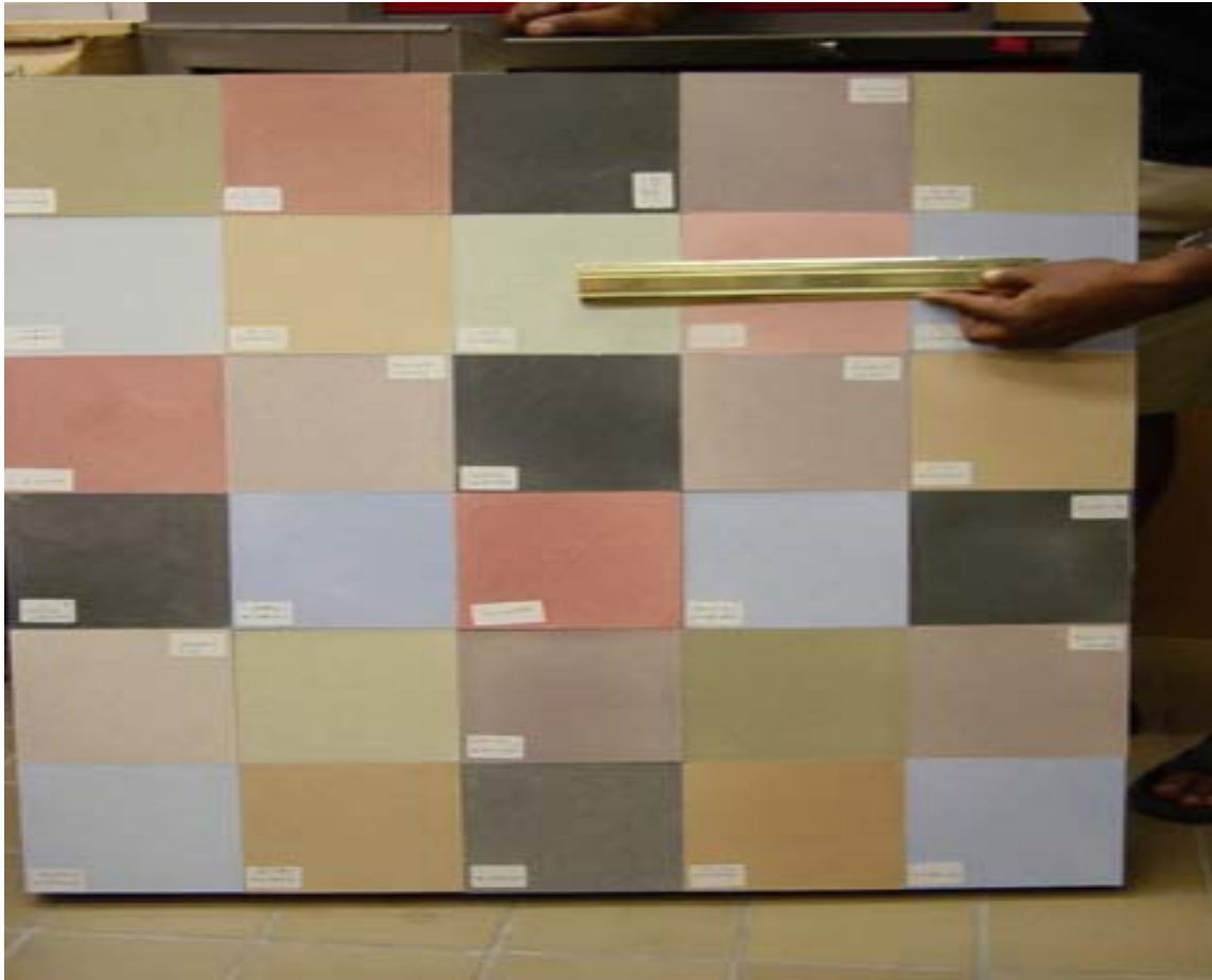
Figure 25. Different color tiles, fabricated from sulfate-rich scrubber sludge, were mounted on a commercial Durock board.
