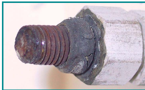
Figure 4.56. Passive probe after service.
