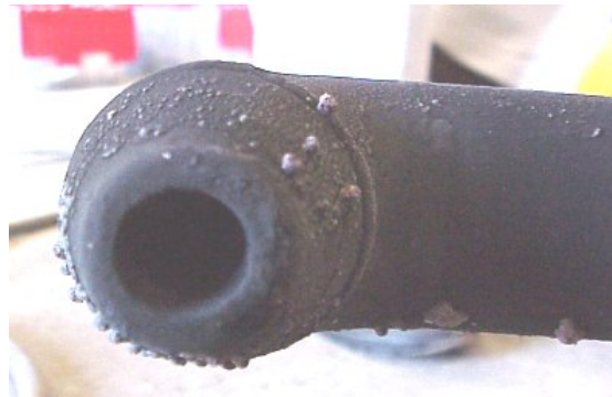
Figure 4.69. Tip of the sampling probe after testing in the pilot-scale facility.
