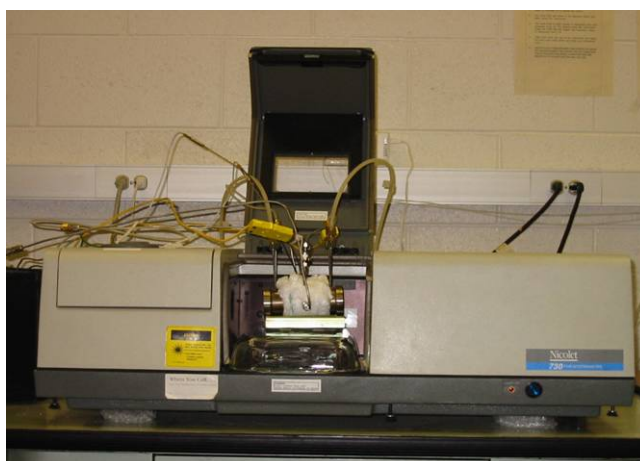
Figure 5.11. FTIR spectrometer with gas cell in sample analysis compartment.
