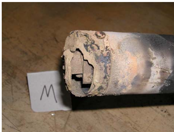
Figure 4.38. Damaged Main Probe illustrating failure due to thermal fatigue.
