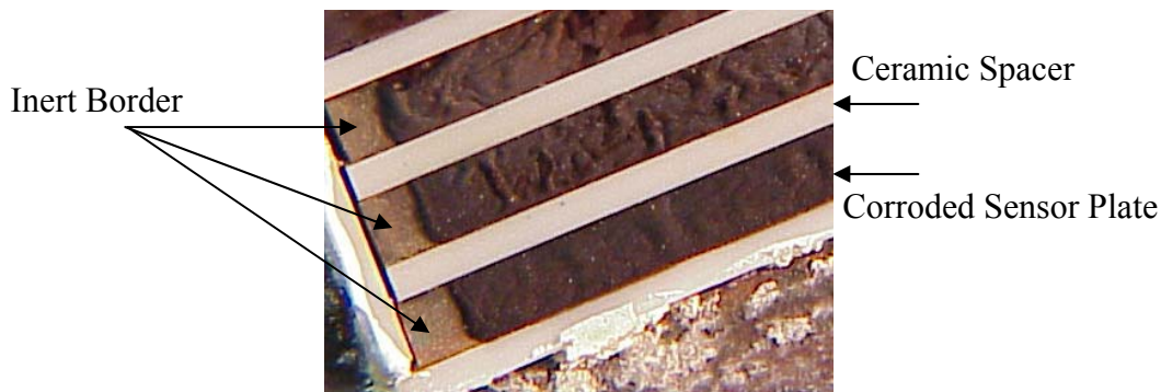
Figure 4.28. The electrochemical sensor array after a corrosion test showing the inert border.
