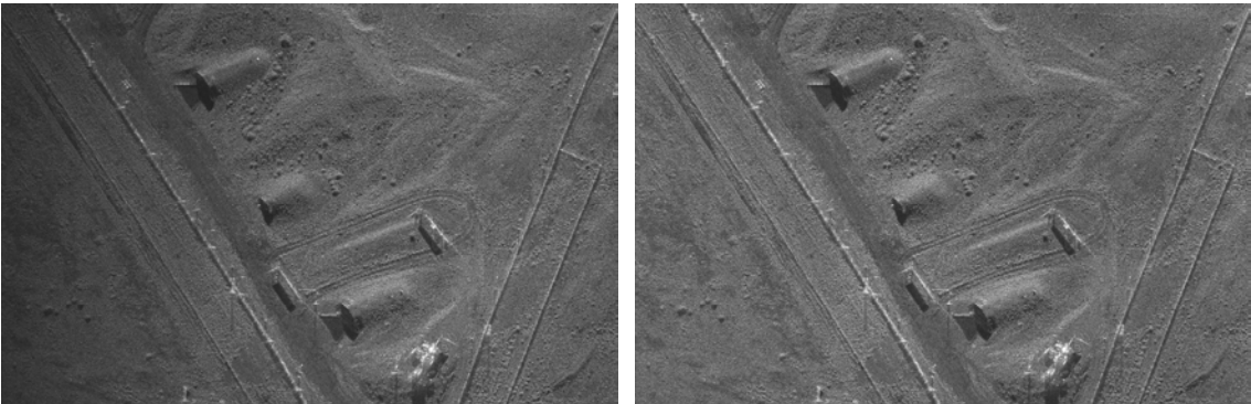
Figure 9. Storage bunker complex. (Ku-band, 0.1 m resolution, 3.3 km range, 31 degree grazing angle)
