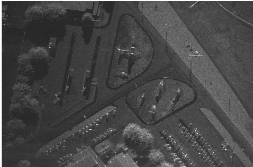
Figure 1. SAR image of static aircraft display exhibiting antenna illumination roll-off on left side (Ku-band, 0.1 m resolution, 3.2 km range, 31 degree grazing angle)
