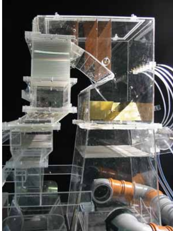
Figure 8. Photograph of the physical flow model used to design the in-duct SCR for AES Greenidge Unit 4 (courtesy of Ruscheweyh Consult GmbH).
