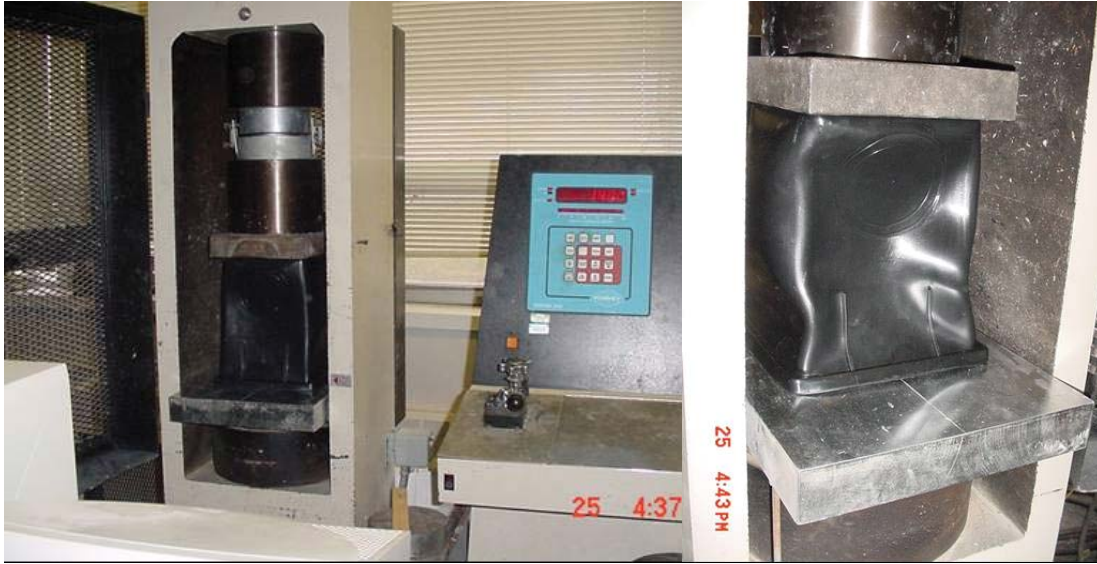
Figure 3-8: Stress test conducted on the leachate sampling basins
