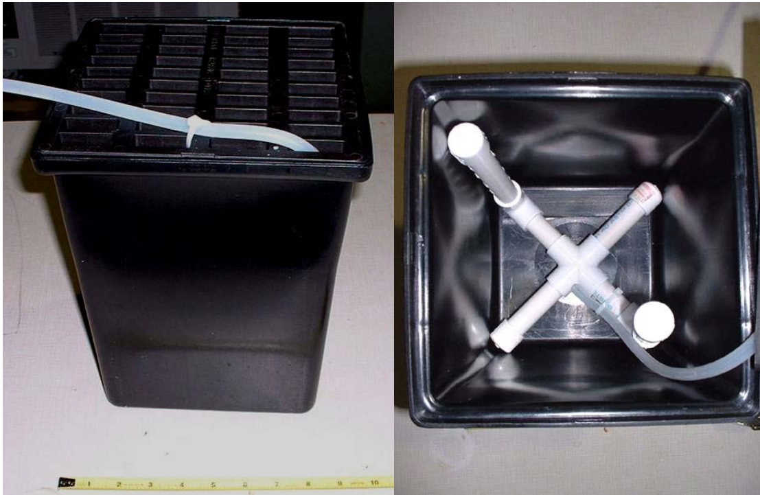
Figure 3-7: Leachate sampling basin
