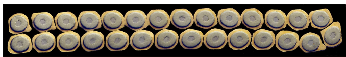
Fig. 4. The Cross-section of a rectangular Ta matrixed F4 Nb 3 Al Rutherford cable with a high compaction factor 86.5 %. Dimensions: 13.95 mm x 1.85 mm.
