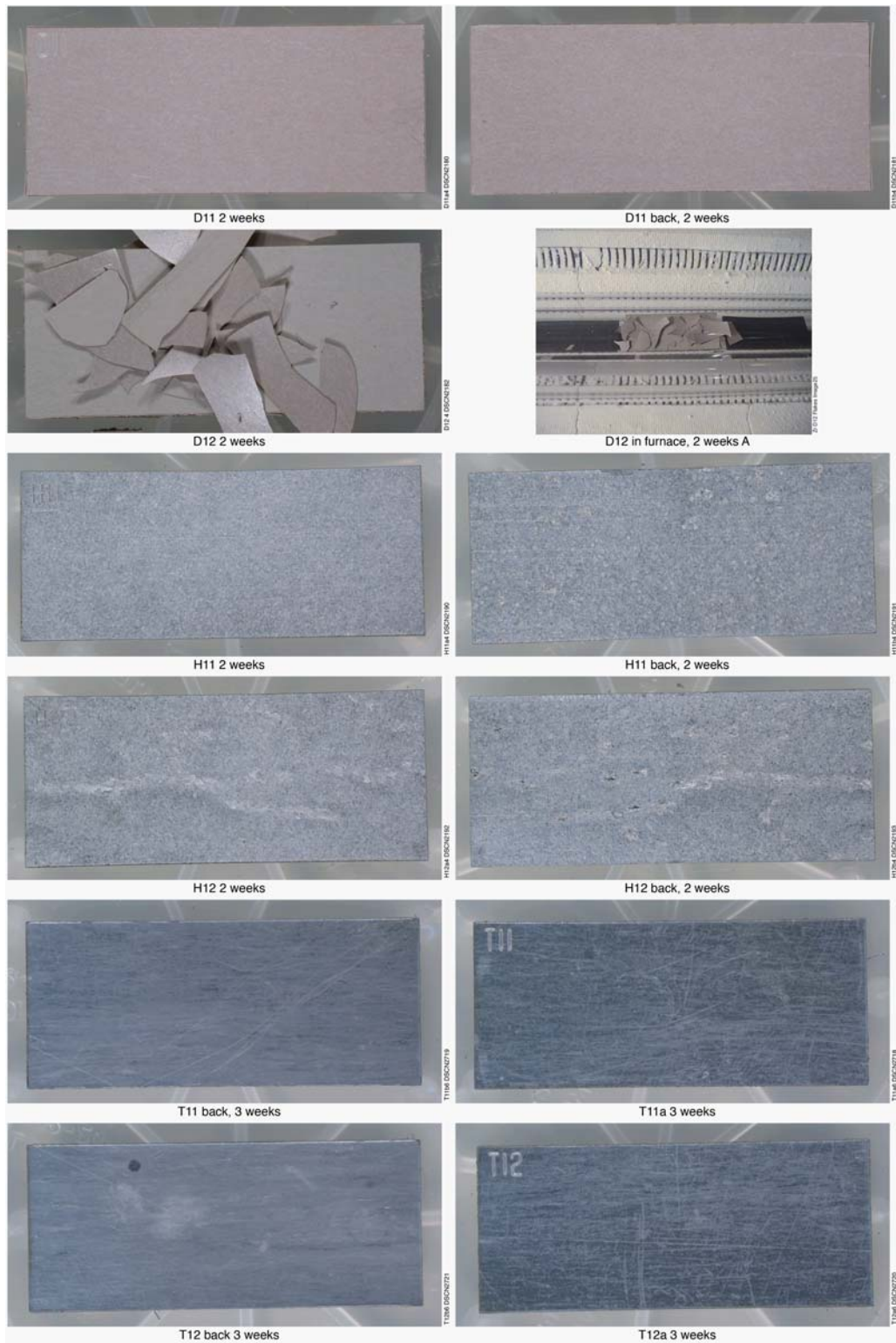
Figure 12. Surface appearance of 4x17 mm coupons of Alloy D (1% Ti) and Alloys H and T (2% Ti, 0.5% Ni). D is shown with its oxide both out of and in the quartz tube in the open furnace. The oxide has flaked off in very coherent sheets that, although some have “landed” on neighboring samples, were easy to retrieve and weigh.
