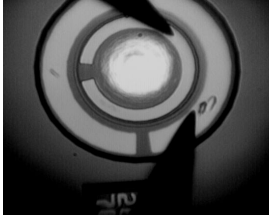
Figure 2.2. Top view microscope photograph of a partially fabricated photodiode being illuminated with an 850-nm laser spot inside the 70- \mu\text{m} top metal aperture.
