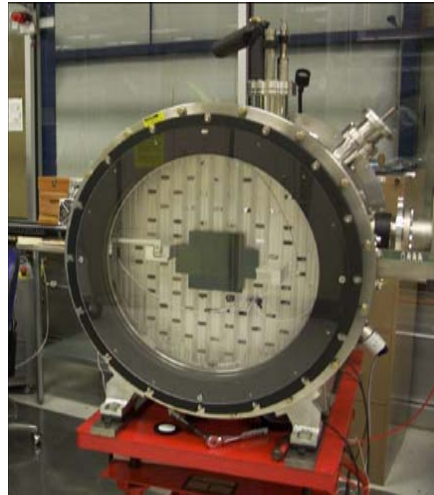
Figure 8. Multi-CCD Test Vessel with the 10 CCD engineering grade mosaic.
