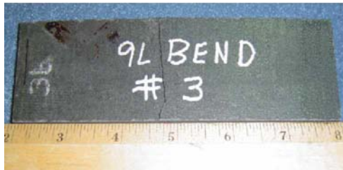
Specimen 3 (side view showing crack)
