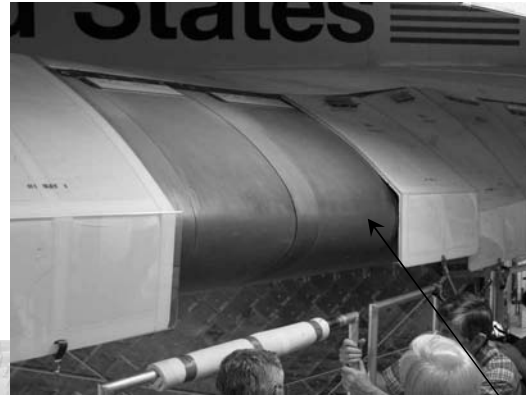
Upper RCC with large overhang from work platform
