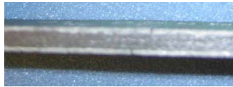
Specimen 1 (side view showing crack)
