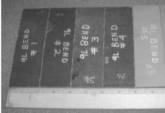
RCC Specimen Undergoing 3 Pt. Bend Test
