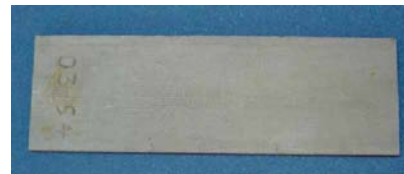
Flaws are flat bottom holes and side slots across width of specimen
