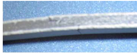
Specimen 3 (side view showing crack)
