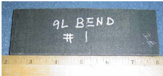
Specimen 1 (side view showing crack)
