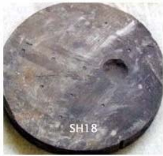
Figure A-60 Sample SH 18A: Laser Parameters: E=4kW, L=1msec, R=200/sec, t=0.5 sec, beam diameter=0.5"
