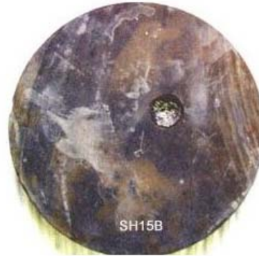
Figure A-58 Sample SH 15B: Laser Parameters: E=4kW, L=1msec, R=400/sec, t=0.5sec, beam diameter=0.375"
