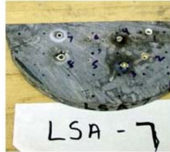
Figure A-36 Sample LSA-7, shots 1-8: Shots 1-6: Laser Parameters: E=8kW, L=1msec, Shots 1 & 2: R=200/sec Shot 1: t=0.5 sec, beam diameter=0.125" Shot 2: t=1.0 sec, beam diameter=0.125" Shots 3-6: R=100/sec Shot 3: t=0.5 sec, beam diameter=0.125" Shot 4: t=1.0 sec, beam diameter=0.125" Shot 5: t=0.5 sec, beam diameter=0.063" Shot 6: t=1.0 sec, beam diameter=0.063" Shots 7 & 8: E=8kW, L=1msec, R=200/sec Shot 7: t=0.5 sec, beam diameter=0.063" Shot 8: t=1.0 sec, beam diameter=0.063"
