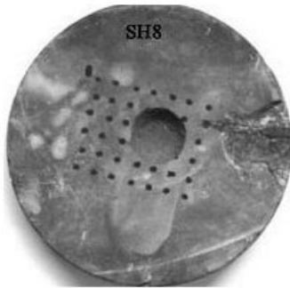
Figure A-47 Sample SH 8: Laser Parameters: E=8kW, L=1msec, R=100/sec, t=0.5 sec, beam diameter=0.5"
