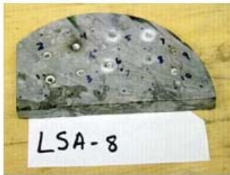
Figure A-37 Sample LSA-8, shots 1-10: Laser Parameters: E=8kW, L=1msec Shots 1 and 2: R=200/sec Shot 1: t=1.0 sec, beam diameter=0.125" Shot 2: t=0.5 sec, beam diameter=0.125" Shots 3-6: R=100/sec Shot 3: t=1.0 sec, beam diameter=0.125" Shot 4: t=0.5 sec, beam diameter=0.125" Shot 5: t=0.5 sec, beam diameter=0.063" Shot 6: t=1.0 sec, beam diameter=0.063" Shots 7-10: R=50/sec Shot 7: t=1.0 sec, beam diameter=0.063" Shot 8: t=0.5 sec, beam diameter=0.063" Shot 9: t=0.5 sec, beam diameter=0.125" Shot 10: t=1.0 sec, beam diameter=0.125
