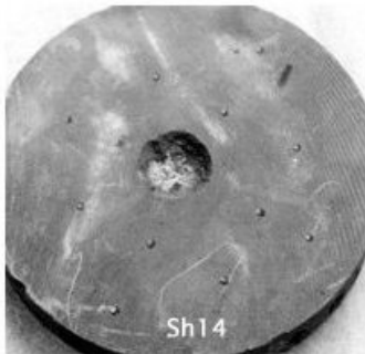
Figure A-55 Sample SH 14: Laser Parameters: E=8kW, L=2msec, R=50/sec, t=1.0 sec, beam diameter=0.5"
