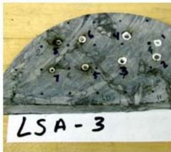
Figure A-33 Sample LSA-3, shots 1-8 Laser Parameters: E=4kW. L=1msec, Shots 1-6: R=400/sec Shots 1 & 2: t=0.5 sec, beam diameter=0.125" Shot 3: t=1.5 sec, beam diameter=0.125" Shot 4: t=1.0 sec, beam diameter=0.125" Shot 5: t=0.5 sec, beam diameter=0.063" Shot 6: t=1.0 sec, beam diameter=0.063 Shots 7 & 8: R=200/sec Shot 7: t=0.5 sec, beam diameter=0.063 Shot 8: t=1.0 sec, beam diameter=0.063
