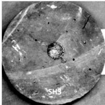
Figure A-41 Sample SH 3: Laser Parameters: E=8kW, L=1msec, R=200/sec, t=0.5 sec, beam diameter=0.375"
