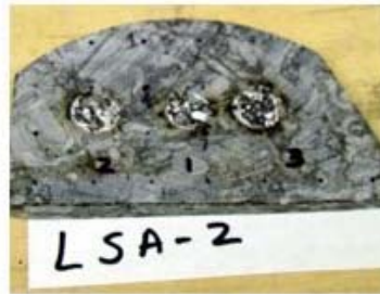
Figure A-32 Sample LSA-2, shots 1 and 2 Laser Parameters: E=8kW. L=1msec, R=200/sec, t=0.5 sec, beam diameter=0.5"
