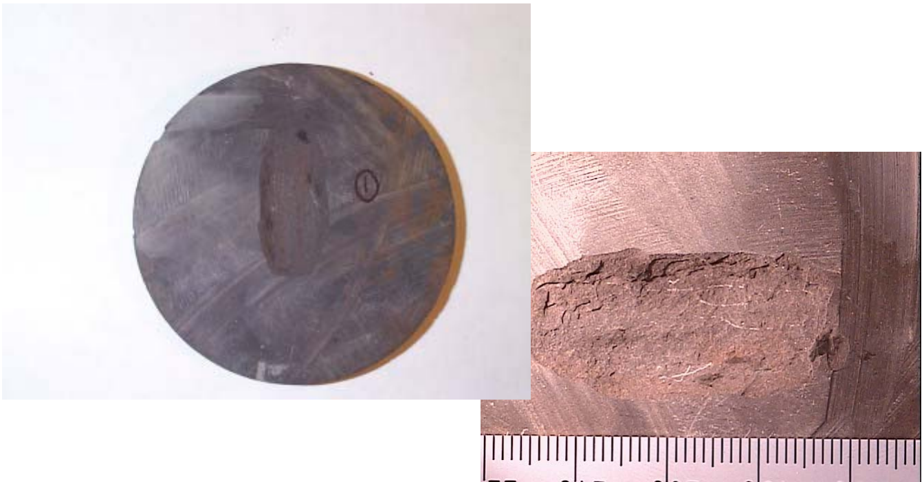
Figure 14. Two views of a shale sample exposed to the Nuvonyx diode laser. The roughly rectangular beam shape can be seen (the sample was stationary during the test). This sample is the opposite face of sample SH8, the lowest SE result of any Nd:YAG test in the dry sample series. It also was the lowest SE of the diode tests.
