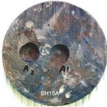
Figure A-57 Sample SH 15A1&A2: Laser Parameters: E=4kW, L=1msec, R=400/sec, t=0.5sec, beam diameter=0.5"
