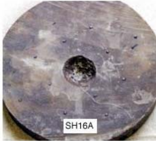
Figure A-59 Sample SH 16A: Laser Parameters: E=4kW, L=1msec, R=400/sec, t=0.5sec, beam diameter=0.5"
