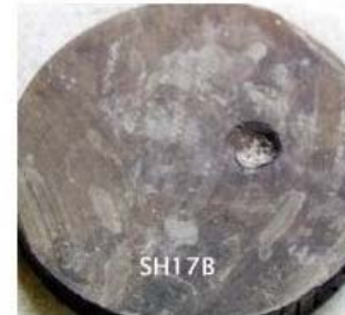
Figure A-62 Sample SH 17B: Laser Parameters: E=4kW, L=1msec, R=200/sec, t=1.0 sec, beam diameter=0.375"
