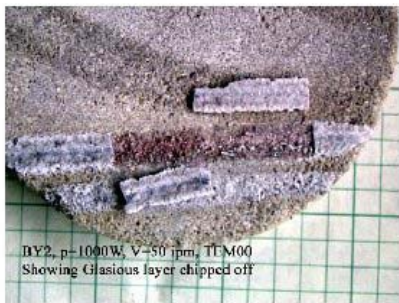
Figure 3c: Berea Yellow SS exhibiting thin glass melt tracks manually removed after exposure to 6kW CO 2 laser in Super Pulsed Mode
