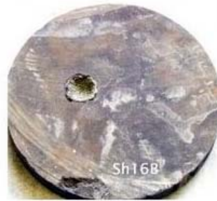
Figure A-60 Sample SH 16B: Laser Parameters: E=4kW, L=1msec, R=400/sec, t=1.0sec, beam diameter=0.375"
