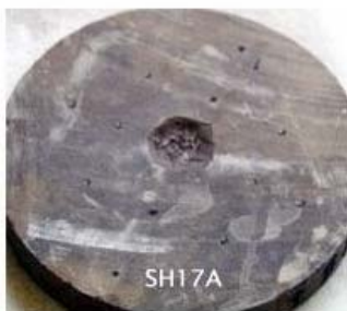
Figure A-61 Sample SH 17A: Laser Parameters: E=4kW, L=1msec, R=200/sec, t=1.0sec, beam diameter=0.5"
