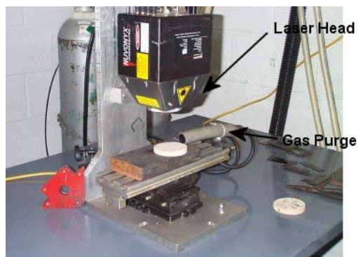
Figure 8. Nuvonyx diode laser system showing sample test configuration.
