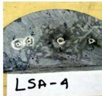
Figure A-34 Sample LSA-4, shots 1-4 Laser Parameters: E=8kW. L=2msec, R=100/sec Shot 1: t=1.5 sec, beam diameter=0.125" Shot 2: t=1.3 sec, beam diameter=0.0625" Shot 3: t=1.0 sec, beam diameter=0.0625" Shot 4: t=1.25 sec, beam diameter=0.0625"
