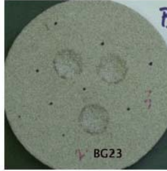
Figure A-20 Sample BG-23, shots 1, 2 and 3. Laser Parameters E=8kW. L=1msec, R=200/sec, t=0.5 secs, beam diameter=0.5"
