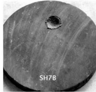
Figure A-46 Sample SH 7B: Laser Parameters: E=8kW, L=2msec, R=100/sec, t=1.0 sec, beam diameter=0.375"
