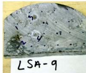
Figure A-38 Sample LSA-9, shots 1-14: Laser Parameters: E=8kW, L=2msec, R=25/sec Shot 1: t=1.0 sec, beam diameter=0.125" Shot 2: t=0.5 sec, beam diameter=0.125" Shot 3: t=0.5 sec, beam diameter=0.063" Shot 4: t=1.0 sec, beam diameter=0.063"
