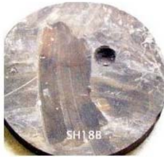
Figure A-61 Sample SH 18B: Laser Parameters: E=4kW, L=1msec, R=200/sec, t=0.5 sec, beam diameter=0.375"
