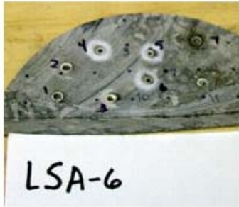
Figure A-35 Sample LSA-6, shots 1-8 Laser Parameters: E=8kW, L=2msec, Shots 1-4: R=100/sec Shot 1: t=0.5 sec, beam diameter=0.125" Shot 2: t=1.0 sec, beam diameter=0.125" Shot 3: t=1.0 sec, beam diameter=0.0625" Shot 4: t=1.25 sec, beam diameter=0.0625" Shots 5-8: R=50/sec Shot 5: t=1.0 sec, beam diameter=0.0625" Shot 6: t=0.5 sec, beam diameter=0.063 Shot 7: t=0.5 sec, beam diameter=0.125 Shot 8: t=1.0 sec, beam diameter=0.125
