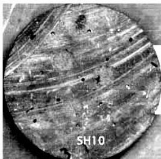
Figure A-49 Sample SH 10: Laser Parameters: E=8kW, L=1msec, R=50/sec, t=0.5 sec, beam diameter=0.5"
