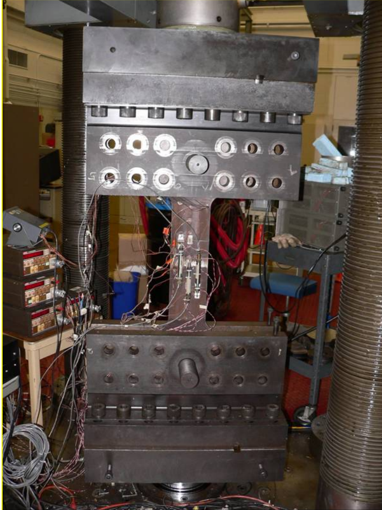
Figure 3-37 A mini-wide-plate specimen with the instrumentation
