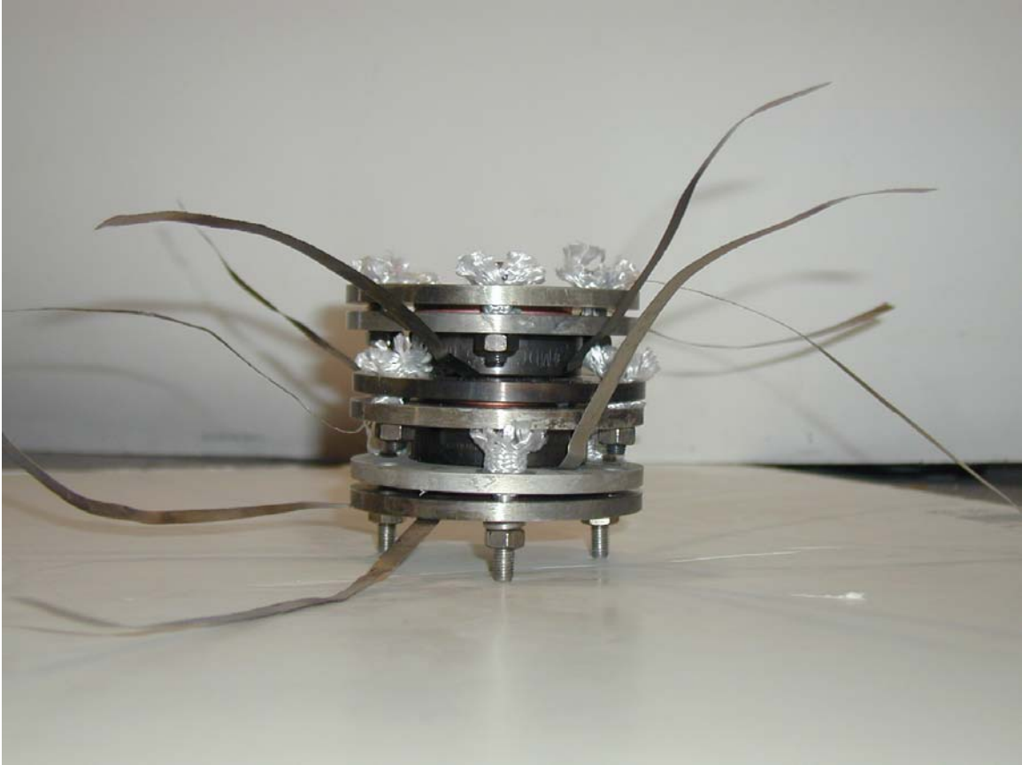
Figure 27: The planar three cell stack assembly used for testing.
