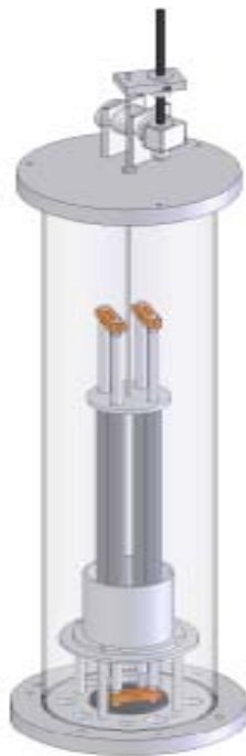
Figure 11: The motor-driven mechanism to position the wick assembly
