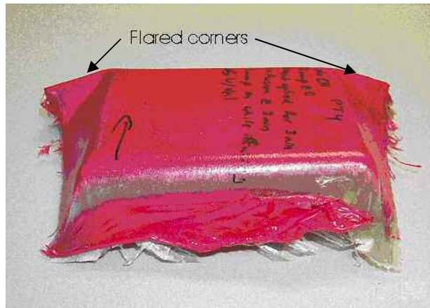
Figure 6. Part with flared corners.
