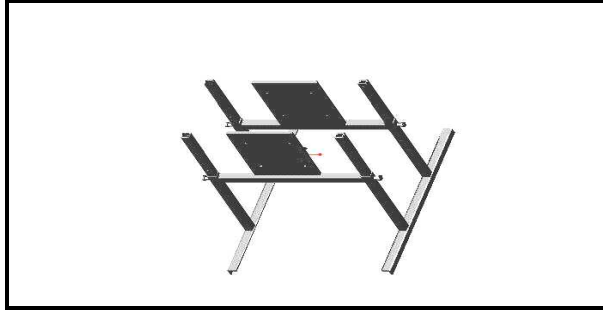
Figure 23. 3D schematic representation of the UV lamp support stand.
