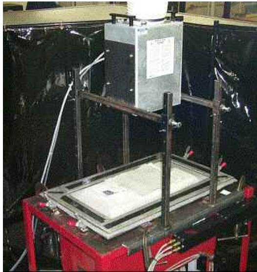
Figure 24. UV Lamp mounted over the RIDFT.
