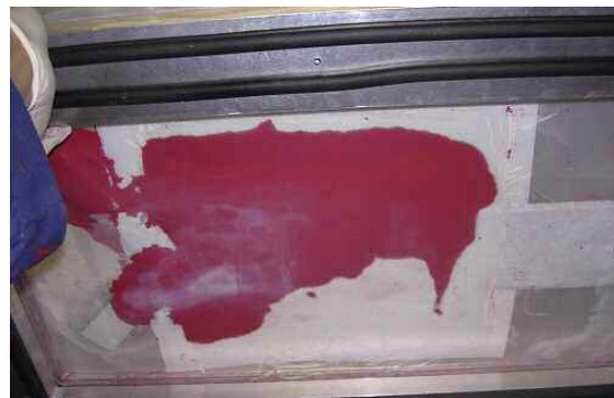
Figure 16. (a) Coating material in contact with FERRO #MCO8 Prepak™ separation material; (b) Depletion of separation layer after 60 seconds.
