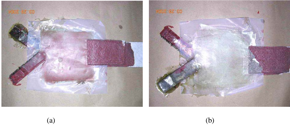
Figure 14. (a) Top (coating) side of coinfused component; (b) Bottom (resin) side of component.
