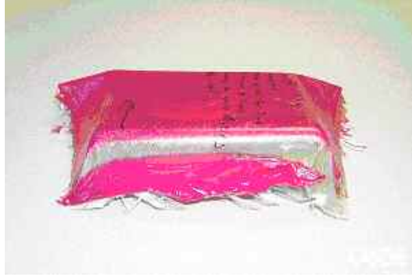
Figure 9. Part with paint separation.
