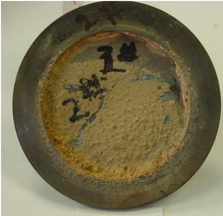
coupon after test at water wall 160 hr (coal )
