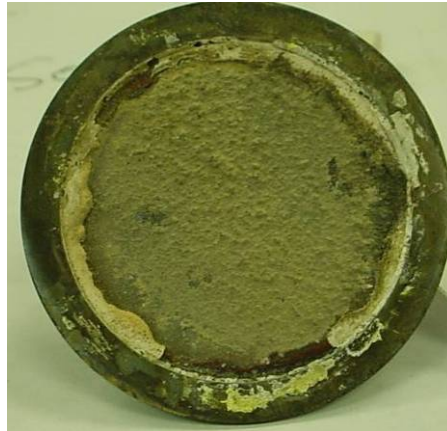
coupon after test at waterwall, 28 hr (biomass, then coal)
