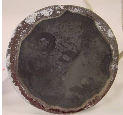
coupon after test at superheater, 8 hr coal then biomas
