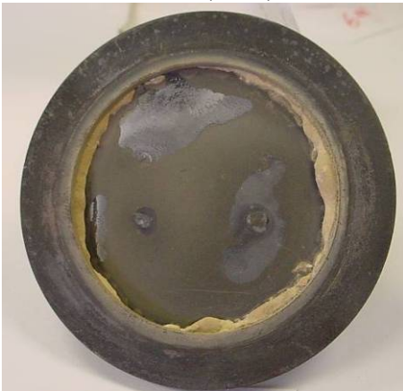
coupon after test at superheater, 50 hr biomass
