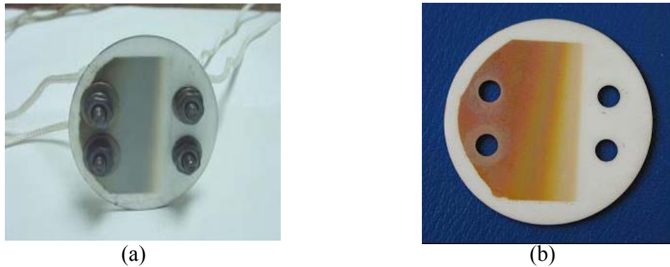
Fig. 2: Pictures of a fabricated sensor, (a) before corrosion (b) after corrosion.
