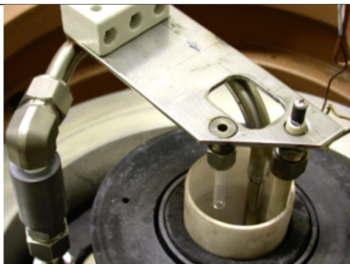
Figure 4.4 Second generation of feedthrus on elevator
