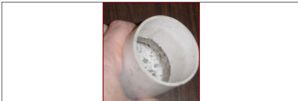
Figure 4.5 Slag on walls of crucible after melting and freezing reagent-grade LiCl-KCl
