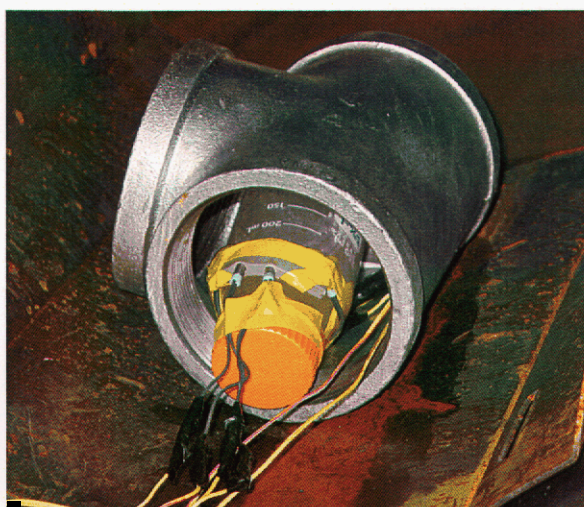
Figure 7. Flask of B. thuringiensis fitted with deta sheet and four RP-2 EBW detonators, loaded into pipe tee in the EDS vessel
