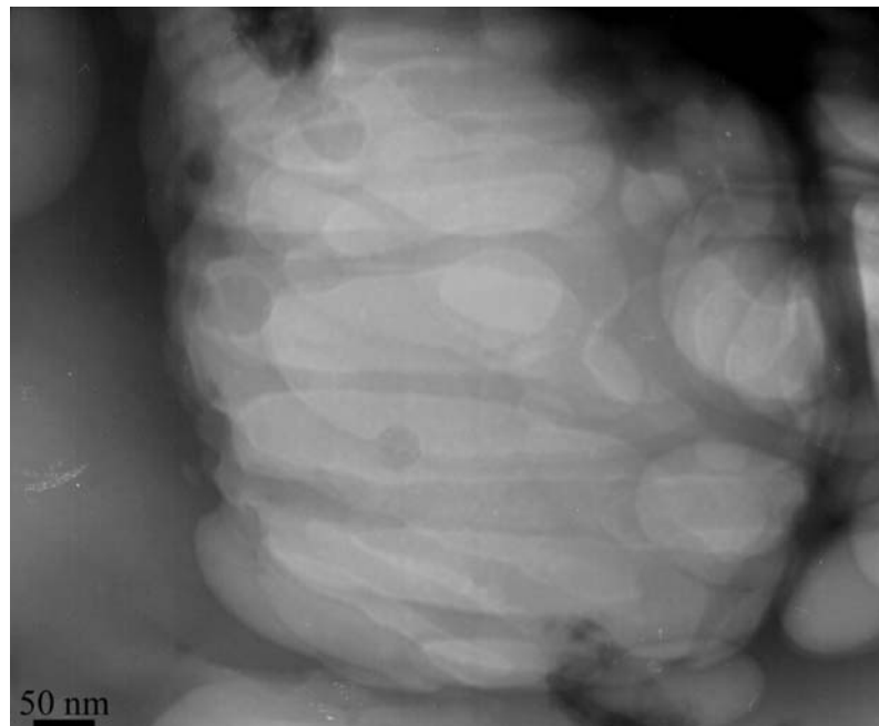
Figure 12. TEM images of porous carbon nanostructures containing nanofibers (propane at a flow rate of 5.40\text{E-}7 \text{ m}^3/\text{s} ).
