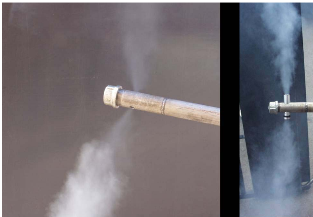
Figure 6. Evaluation of injection lance port designs, simple hole design (left) and nozzle extensions (right). The nozzle extensions provided a more uniform distribution pattern.
