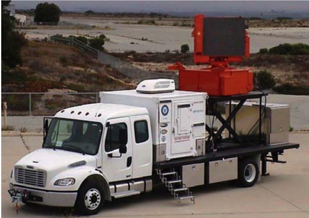
Figure 7. MWR-05XP installed on a heavy-duty truck. The 1.2 m phased array antenna provides electronic beam scanning in elevation and combines electronic back-scanning with mechanical scanning in azimuth.
