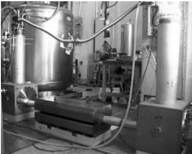
Fig. 8. The 1 m asymmetric model built at KEK. The cooling of the transmission line was made by the liquid flow between supply bottle and outlet bottle.
