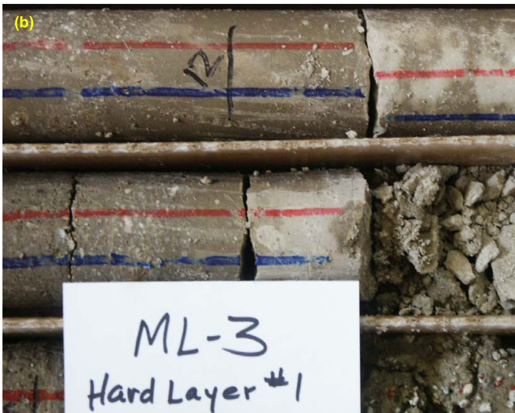
Figure A-14 Photographs of core from the so-called “first hard layer.” (a) Drill hole ML-1, ~13 ft; (b) drill hole ML-3, ~12 ft. Core trays are approximately 2 inches wide.
