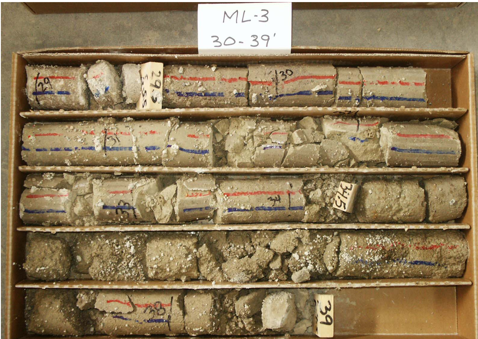
Figure A-12 Photograph of core from drill hole ML-3, 29.0 to 39.0 ft (TD).
