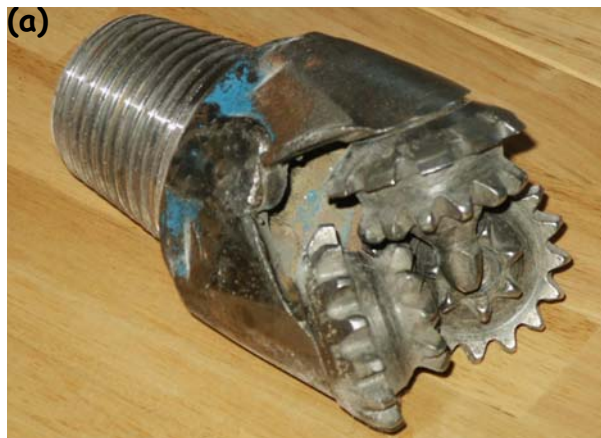
Figure 31. (a) Photograph of a standard tricone drilling bit for use in medium-hard formations; (b) illustration of a drag bit for use in soft and very soft formations.
