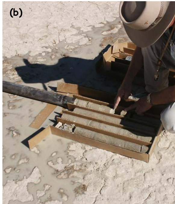
Figure 7. Photographs showing core handing at the rig. (a) Removing core from the inner tube onto a staging rack prior to marking and boxing. (b) Extruding core from the inner tube to avoid excessive disruption of soft or friable core. The inner tube is on the left-hand side of the photograph.
