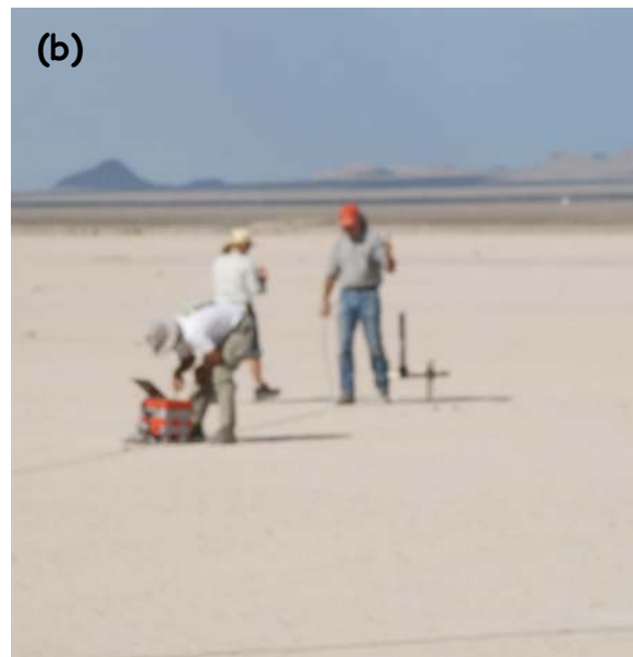
Figure 19. Field TEM measurements. (a) One-half (approximately) of a TEM loop. The transmitter assembly and wire spool are on the left and the central loop system is on the right. (b) Detail of a TEM central-loop layout. The receiver coil is slightly elevated above the lake surface on the right and the recording equipment is inside the orange box on the left.
