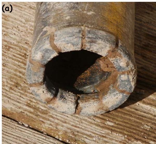
Figure 30. Photographs of different style core bits used during characterization drilling. (a) Diamond-impregnated bit; (b) surface-set diamond bit with stepped design. Overall HQ-size bit diameter is slightly larger than 3-½ inches.
