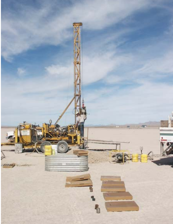
Figure 6. Photographs of core rig in operation of Main Lake. Note core rods and drilling mud.
