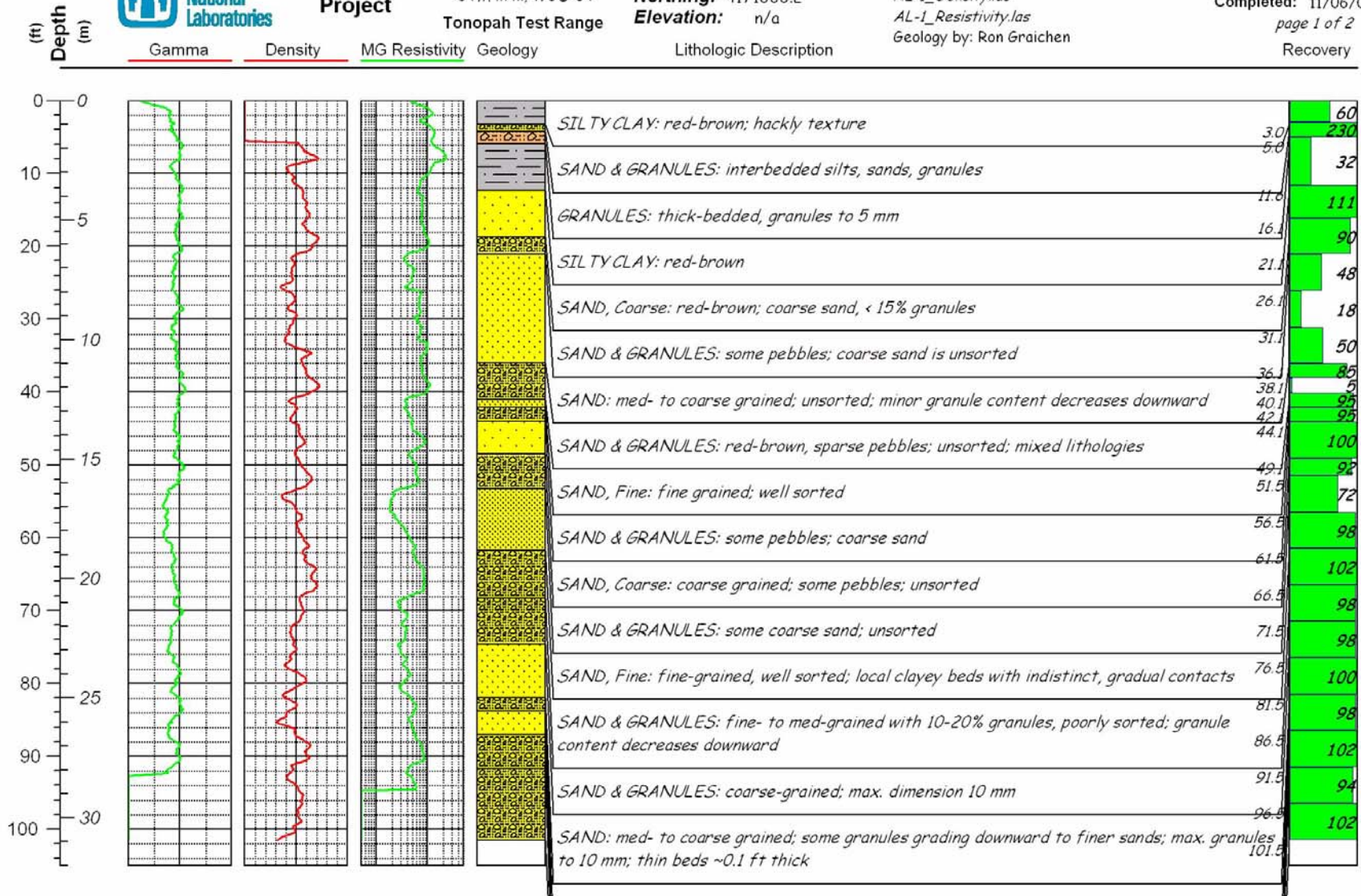
Figure H-1 Geologic core log and geophysical logs for drill hole AL-1.
