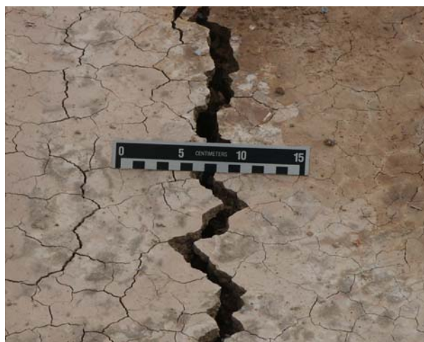
Figure 47. Fracture induced by drilling vibrations extending away from a drill hole on Antelope Lake. (a) Close-up view showing centimeter-scale width of fracture; (b) En-echelon fracture patterns of a drilling-induced fracture (centimeter scale is circled).
