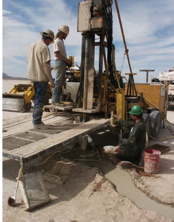
Figure 6. Photographs of core rig in operation of Main Lake. Note core rods and drilling mud.
