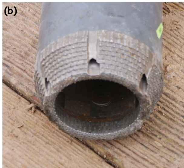
Figure 30. Photographs of different style core bits used during characterization drilling. (a) Diamond-impregnated bit; (b) surface-set diamond bit with stepped design. Overall HQ-size bit diameter is slightly larger than 3-½ inches.
