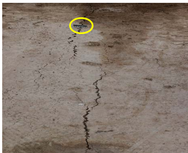
Figure 47. Fracture induced by drilling vibrations extending away from a drill hole on Antelope Lake. (a) Close-up view showing centimeter-scale width of fracture; (b) En-echelon fracture patterns of a drilling-induced fracture (centimeter scale is circled).
