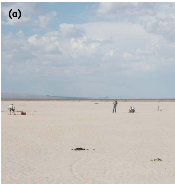
Figure 19. Field TEM measurements. (a) One-half (approximately) of a TEM loop. The transmitter assembly and wire spool are on the left and the central loop system is on the right. (b) Detail of a TEM central-loop layout. The receiver coil is slightly elevated above the lake surface on the right and the recording equipment is inside the orange box on the left.
