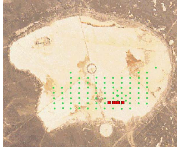
Figure 25. Locations of TEM loops (red squares), Schlumberger sounding (collocated with one of the TEM loops), and pre-existing drill holes (green dots) for the geophysical calibration surveys on Main Lake.
