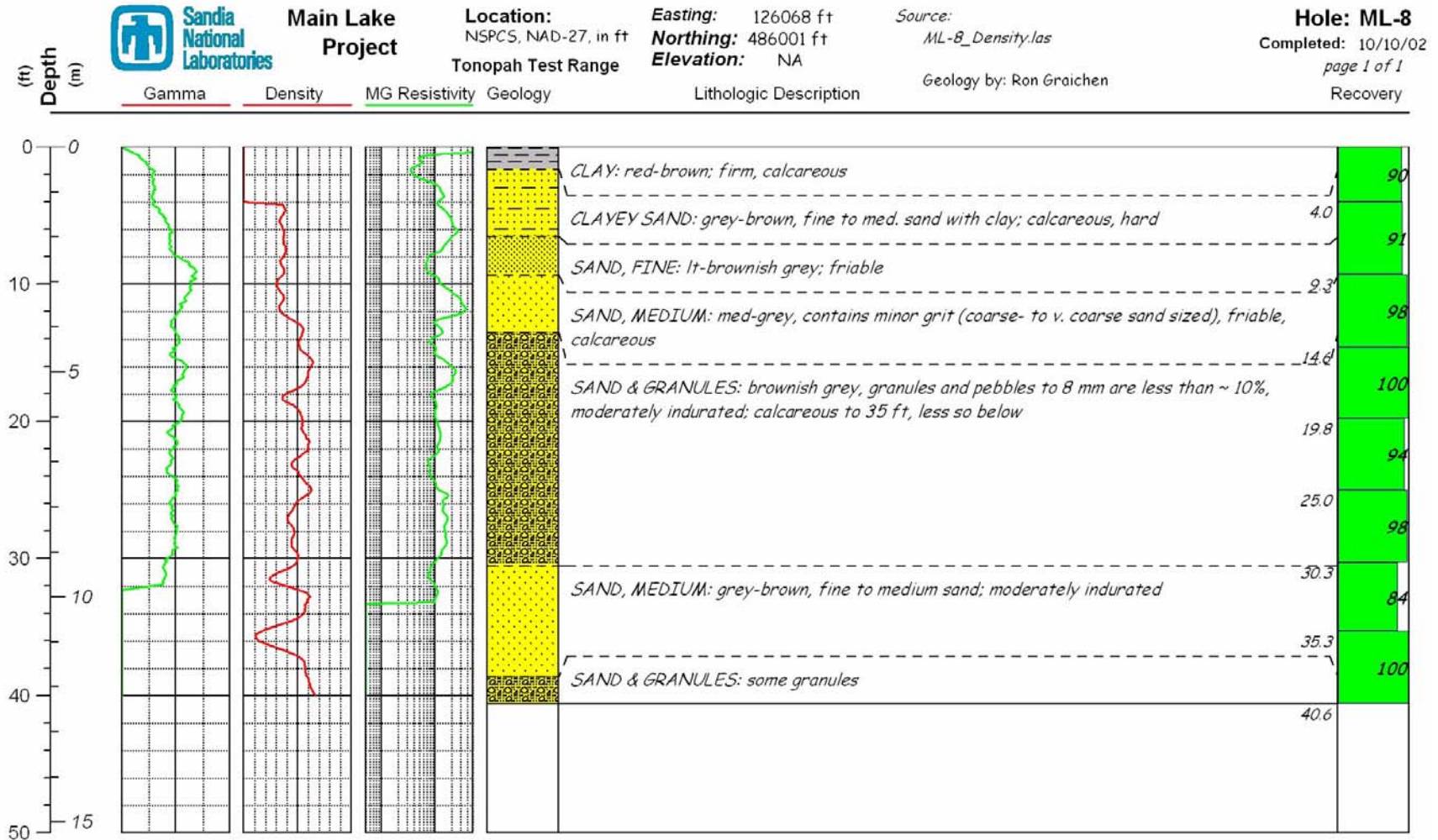
Figure D-8 Geologic core log and geophysical logs for drill hole ML-8.
