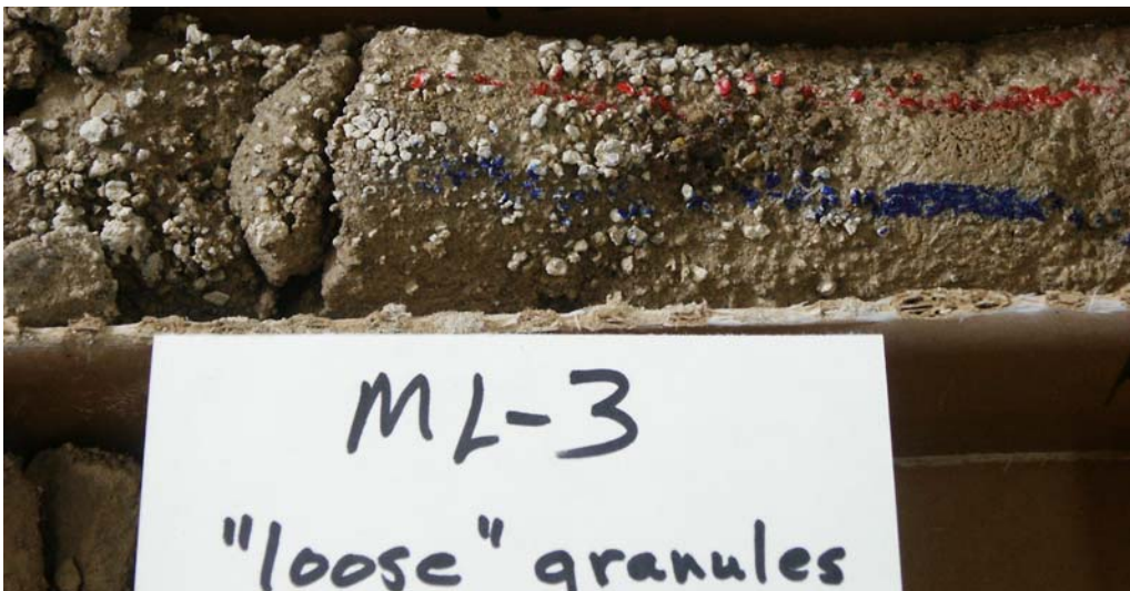
Figure A-18 Photograph showing loose volcanic-clast granules on the surface of an otherwise mud-rich interval of core from drill hole ML-3, ~37 ft.
