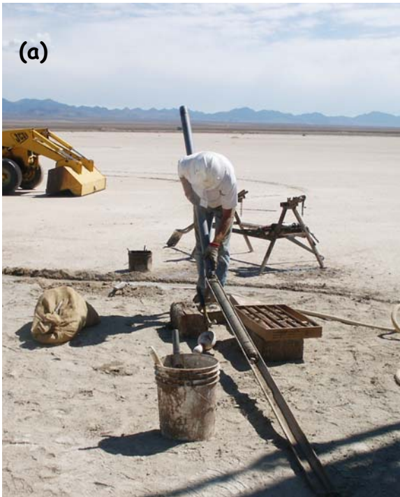
Figure 7. Photographs showing core handing at the rig. (a) Removing core from the inner tube onto a staging rack prior to marking and boxing. (b) Extruding core from the inner tube to avoid excessive disruption of soft or friable core. The inner tube is on the left-hand side of the photograph.
