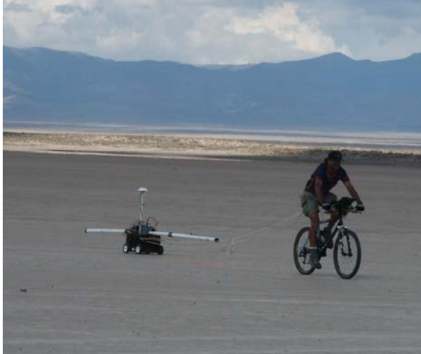
Figure 24. Bicycle-towed EM-31 equipment. Horizontal white cylinder is the Slingram-configured EM transmitter and receiver assembly. Vertical device is GPS receiver. Electronics equipment is inside the cart.
