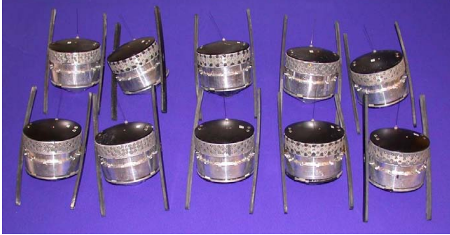
Figure 5: Hopping landmine robots used in self-healing minefield tests.
