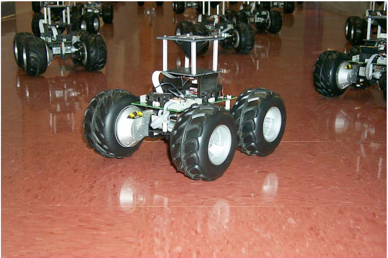
Figure 9: Robot vehicles used in an indoor communication/navigation network.
