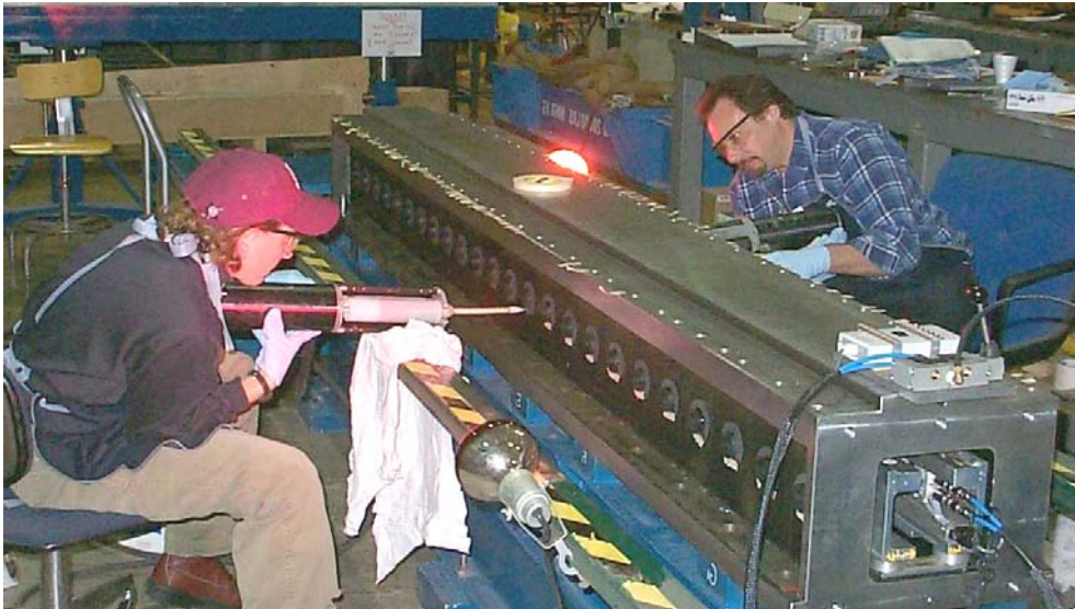
Figure 3, gluing the plastic inserts into the girder. The end of the pneumatic tool which allows high precision to be achieved is visible at the end of the
