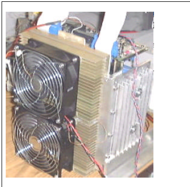
Figure 4-3 Integrated AIPM, Heat Sink and Cooling Fans
