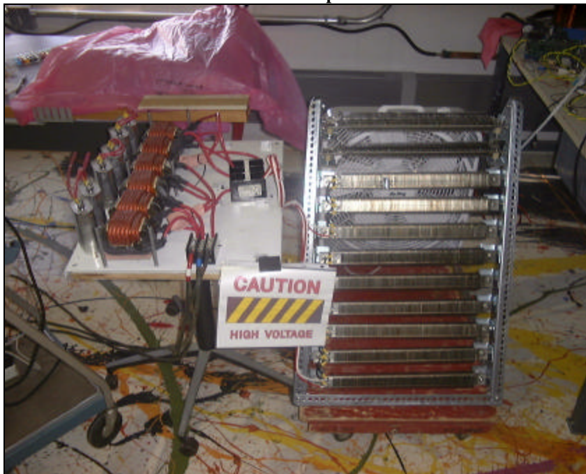
Figure 5.5-5: Inductive and Resistive load bank
