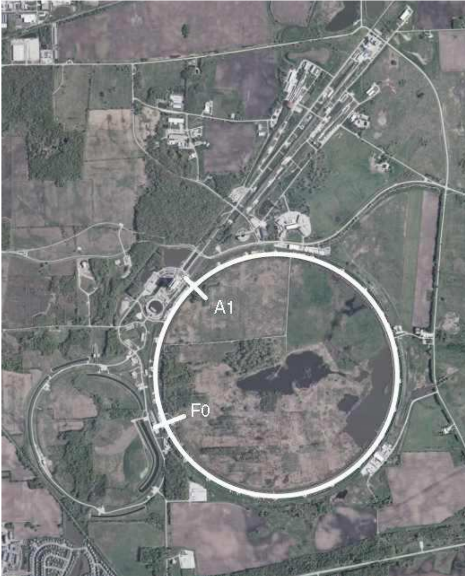
Fig. 3. An aerial view of the Fermilab accelerator complex. The white circle marks the Tevatron which is 2000 m in diameter. The phase modulation is done at house F0 and the CT is at house A1.
