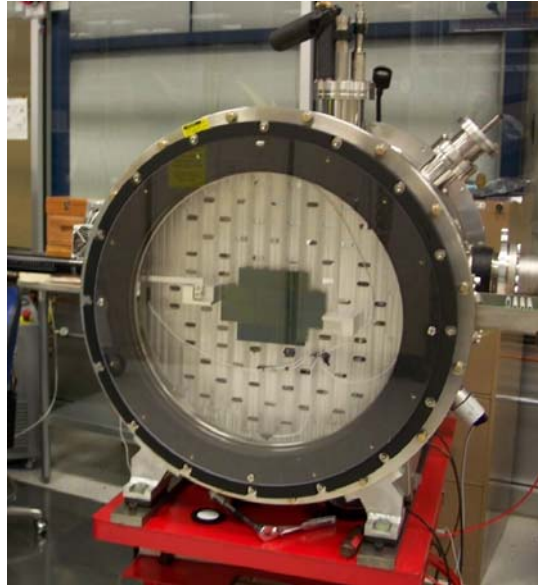
Figure 5-1 The Multi-CCD Test Vessel with 10 2kx4k CCDs mounted on the prototype focal plane support plate.
