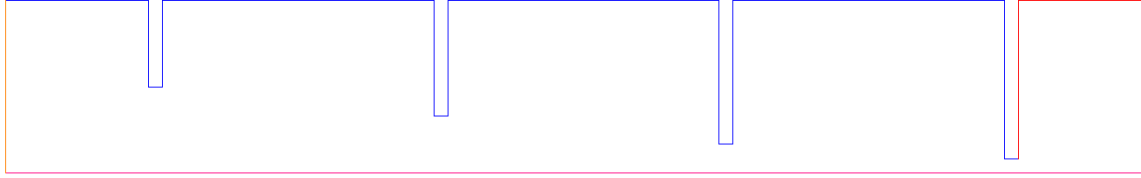
Figure 1. Schematic of a four-stage aerodynamic lens system with orifice.
