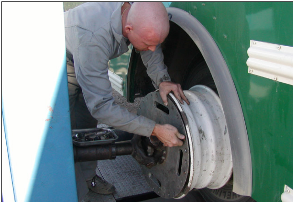
Figure 4: Hub adapters connect the vehicle's drive axle to the power absorber units.
