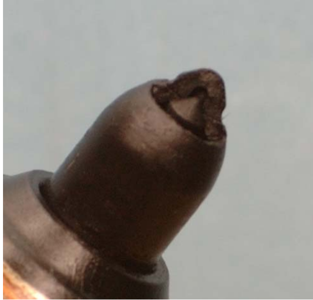
Figure 3: Broken injector tip, showing nozzle sac, and nozzle needle
