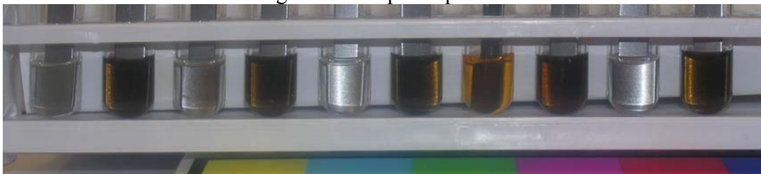
From left to right, S2 Winter, S2 Winter with oil, S2, S2 with oil, S1, S1 with oil, biodiesel, biodiesel with oil, #2 diesel, and #2 diesel with oil
