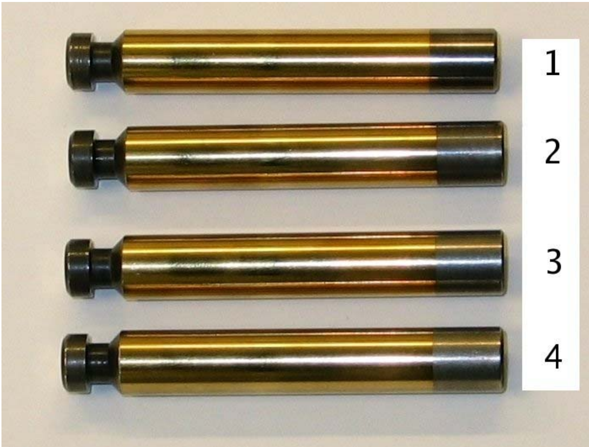
Figure 6. Plungers from the fuel-system durability test engine identified by cylinder number. None show any sign of wear or distress.
