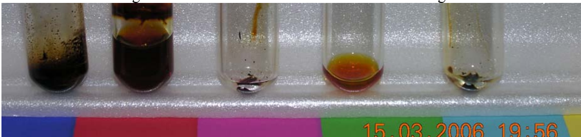
From left to right, conventional diesel, biodiesel, Syntroleum S1 & S2 blend, Syntroleum S2, and Syntroleum S1
