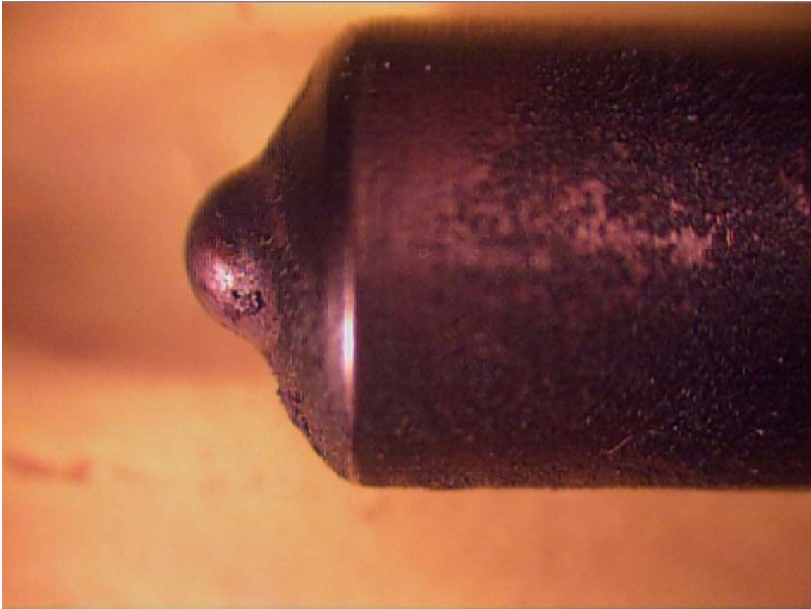
Figure 3.1. Optical microscope image of Caterpillar Injector #3 from AVL 1500 hour durability demonstration showing overall deposit formation in injector tip.
