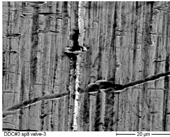
Figure 12. Higher magnification of the rectangular area “on the line” near the center of Figure 11. Although this valve visually “looked” the best of the four, it too had a part of its surface disturbed at some point in its life, but by abrasion, not by the type of adhesive wear that would be caused by insufficient fuel lubricity.
