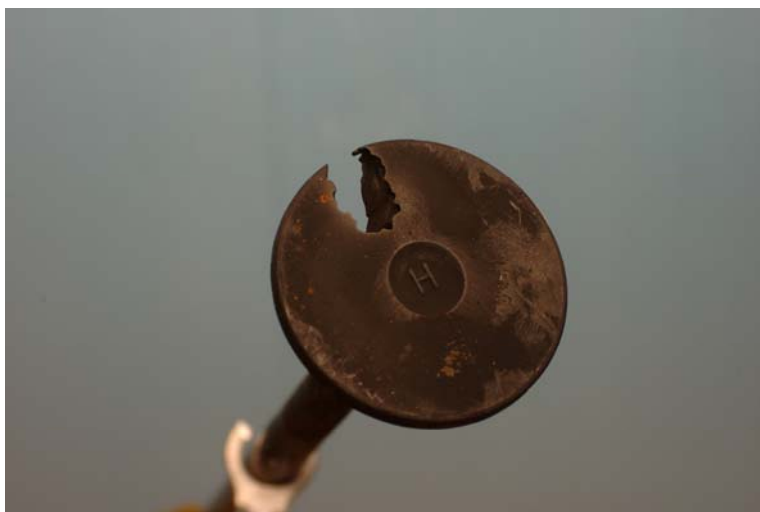
Figure 7: Burned exhaust valve
