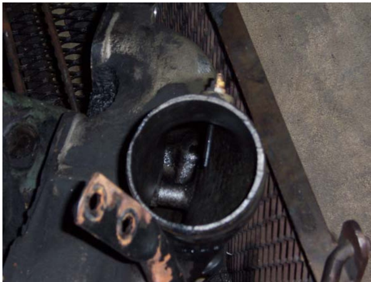
Figure 5: Air Inlet of the intake manifold with crankcase oil from the turbocharger failure
