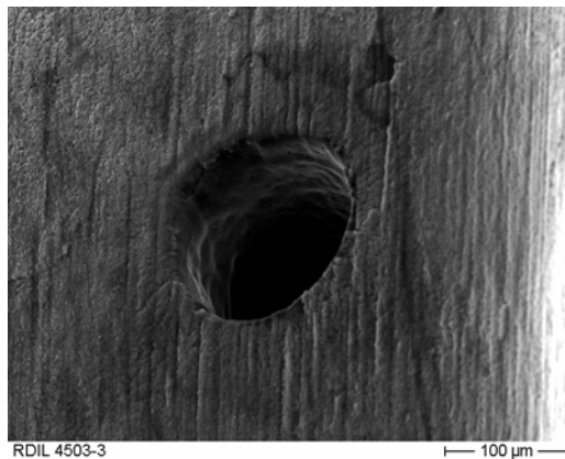
Figure 19: Hole of used nozzle with 104% flowrate of new reference nozzle
