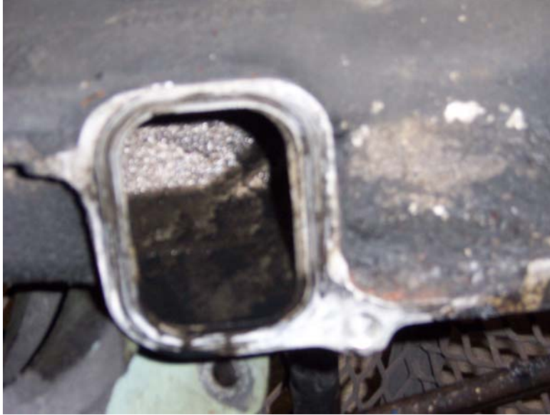
Figure 4: One of the port-connections of the intake manifold with crankcase oil from the turbocharger failure
