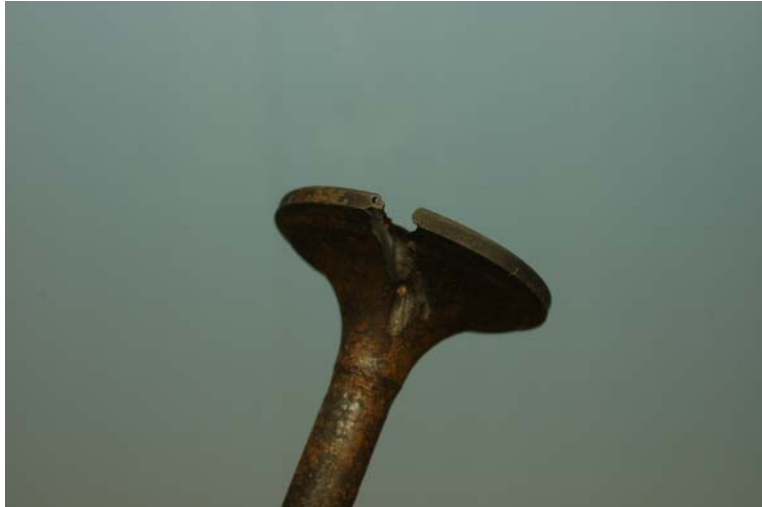
Figure 8: Burned exhaust valve
