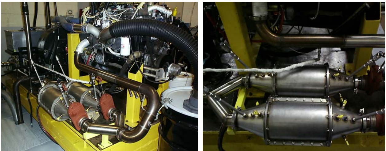
Figure 5.11. Schematic of full-flow trap on test bed. The pressure transducers, flow control valves, and thermocouples are shown in the photographs as well.
