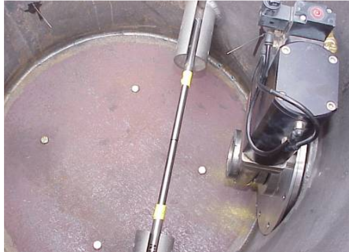
Figure 2.3.2. Phase 2+ Chamber Interior, showing Rodlet, Closure Valve, Thermocouples
