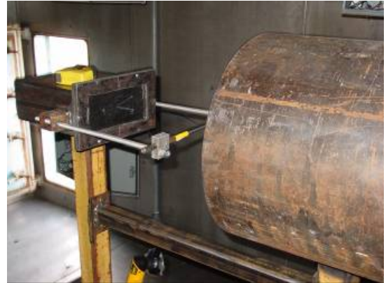
Figure 3.1.5. Test 2/CSC Rodlet and Support Apparatus
