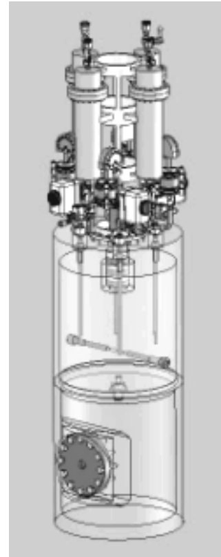
Figure 2.6.1 Diagram of Phase 4 Test Chamber and Aerosol Sampling Systems
