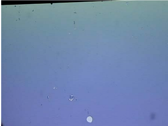
Piece 12: Blank GaAs with 4000 Å \text{SiO}_2 , after RTA (460 °C, 15 s).
