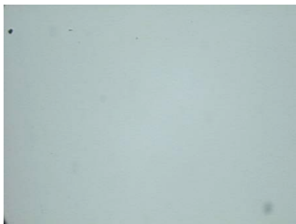
Piece 14: Blank Si with 4000 Å SiO 2 and 200 Ti/ 300 Au, after RTA (460 °C, 15 s).
