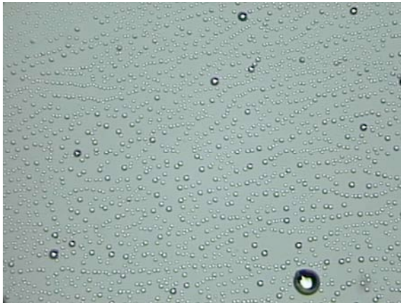
Piece 5: Blank GaAs with 4000 Å SiN x and 200 Ti/ 300 Au, after RTA (460 °C, 15 s).
