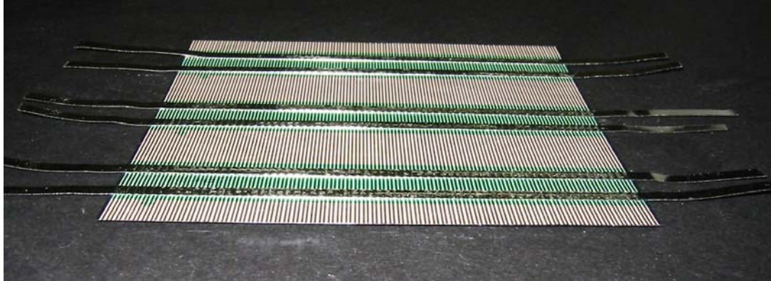
Figure 13. A busbarless cell using conductive adhesive to connect the screen-printed Ag gridlines to the copper ribbon. It exhibits negligible bow compared to a cell with the soldered copper ribbon.
