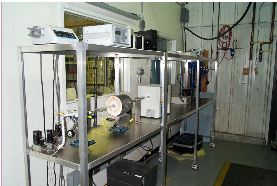
Figure 1.2.1. Arthur D. Little's GENEX-apparatus has been redesigned to operate on diesel fuel
