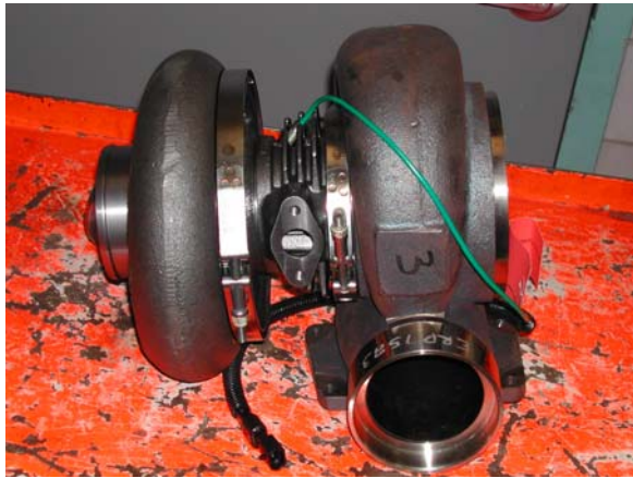
Figure 1.4.2.4: Pictures of (a) low pressure turbocharger and (b) high pressure turbocharger.
