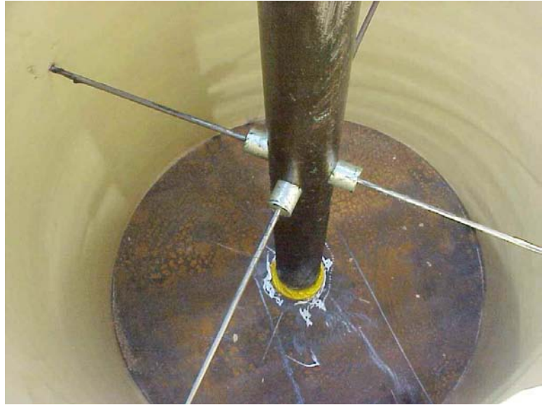
Figure 2. (a) Sonotube form mounted on casting jig (b) Interior of form showing the molds that formed the axial, 4-inch-diameter hole (black tube) and the four fixtures that formed the mounting holes for the accelerometers.
