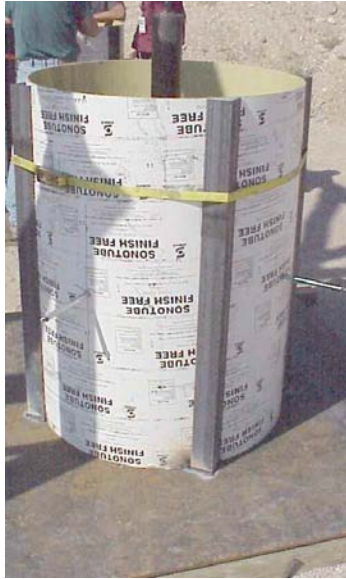
Figure 2. (a) Sonotube form mounted on casting jig (b) Interior of form showing the molds that formed the axial, 4-inch-diameter hole (black tube) and the four fixtures that formed the mounting holes for the accelerometers.
