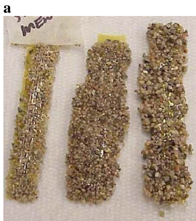
Figure 3. (a) Sand-encapsulated strain gages ready for mounting on the emplacement jig (b) emplacement jig used to hold strain gages at proper radial distances and orientation while pouring the specimen.
