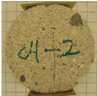
Figure 36. Post-test photograph of a Brazilian test specimen, showing the tensile crack induced by loading along the axis parallel the crack.
