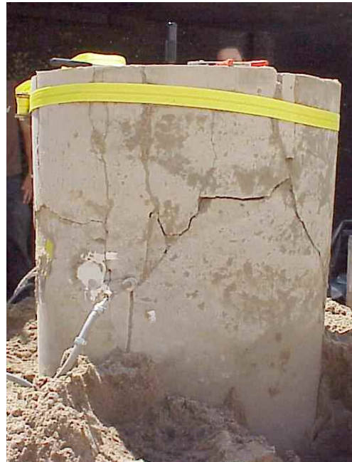
Figure 10. (a) Post-test top view showing radial cracking and near-borehole cratering (b) Post-test side view with specimen stabilized by strap. With radial motion restrained by the sand and culvert, the specimen remained relatively intact.
