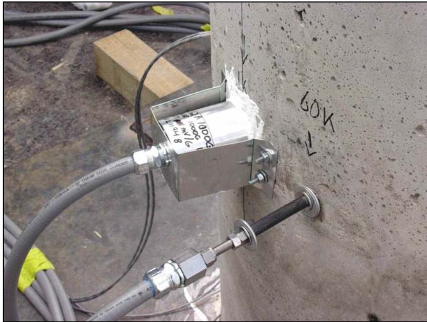
Figure 8. External accelerometer mounted on specimen to the left of the exit point for one of the embedded accelerometers.
