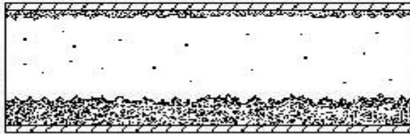
Figure 19 - Annular-Oil Continuous (AN-OC) and Annular -Water Continuous (AN-WC) Gas-Oil-Water Flow Patterns
