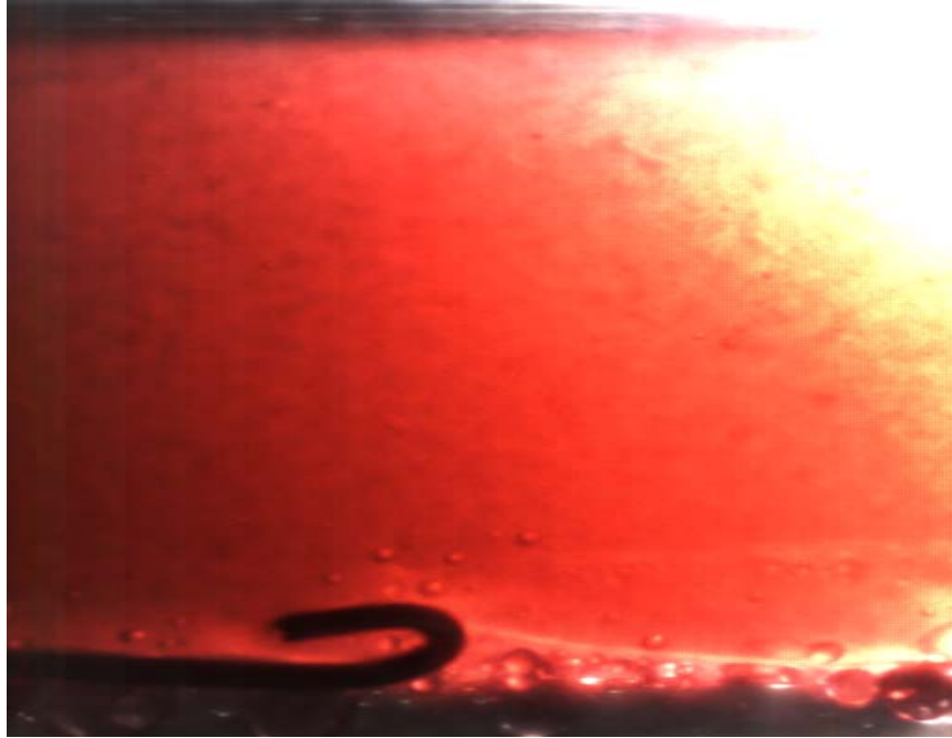
Figure 36 - v_{so}=0.500 m/s v_{sw}=0.025 m/s (DW/O&O)
