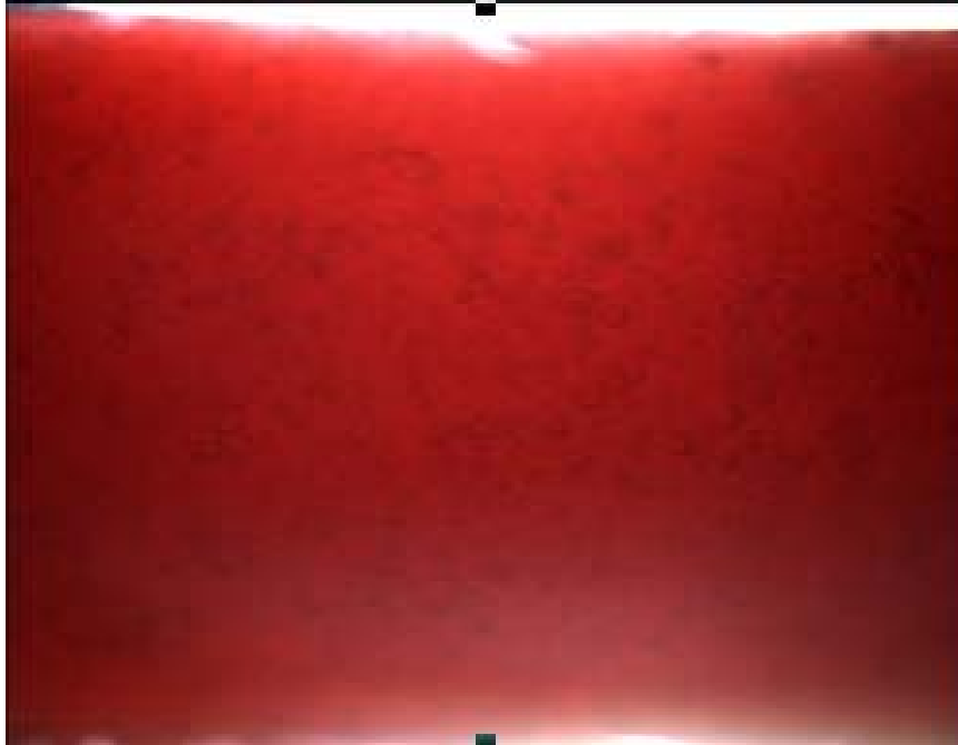
Figure 34 - v_{so}= 1.750 m/s v_{sw}=0.100 m/s (DW/O)
