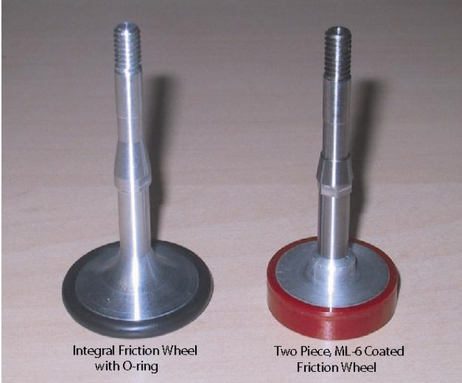
Figure 16. Integral and Two-Piece Friction Wheels Showing Different Friction Materials
