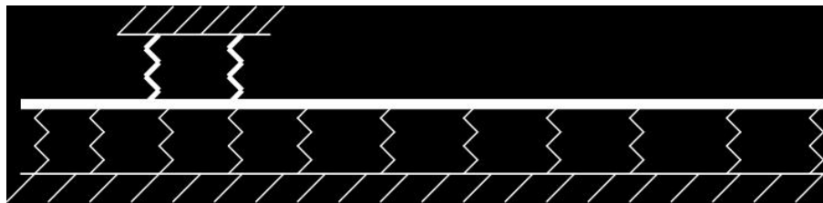
Figure 7. Finite Element Analysis Model Used to Determine the Spindle Design's First Natural Frequency
