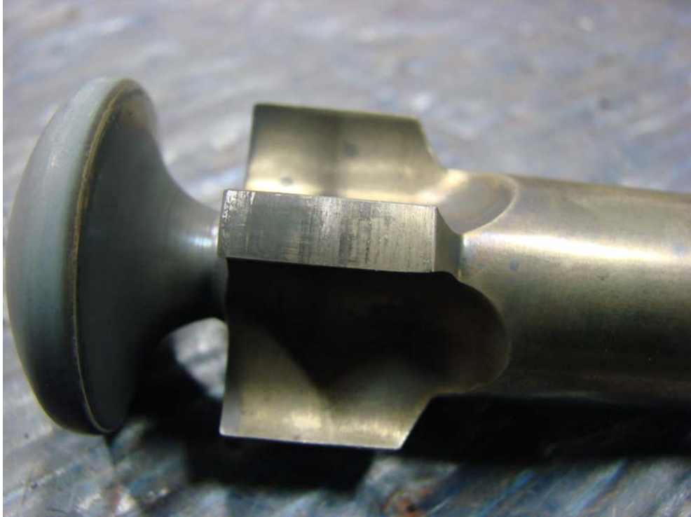
Figure B3: Pressure regulator valve of 316 stainless steel after +1,000,000 cycles of operation in a 316L body in steam at 350°F. Enlarged view of the polishing on the wear surface shows essentially no wear.
