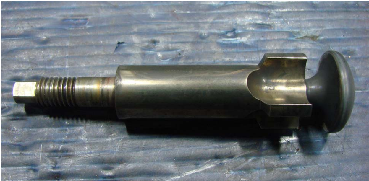
Figure B2: Pressure regulator valve of 316 stainless steel after +1,000,000 cycles of operation in a 316L body in steam at 350°F. Only slight polishing on the wear surfaces on the guide flues was noted. This was called “very impressive” by Spirax Sarco.
