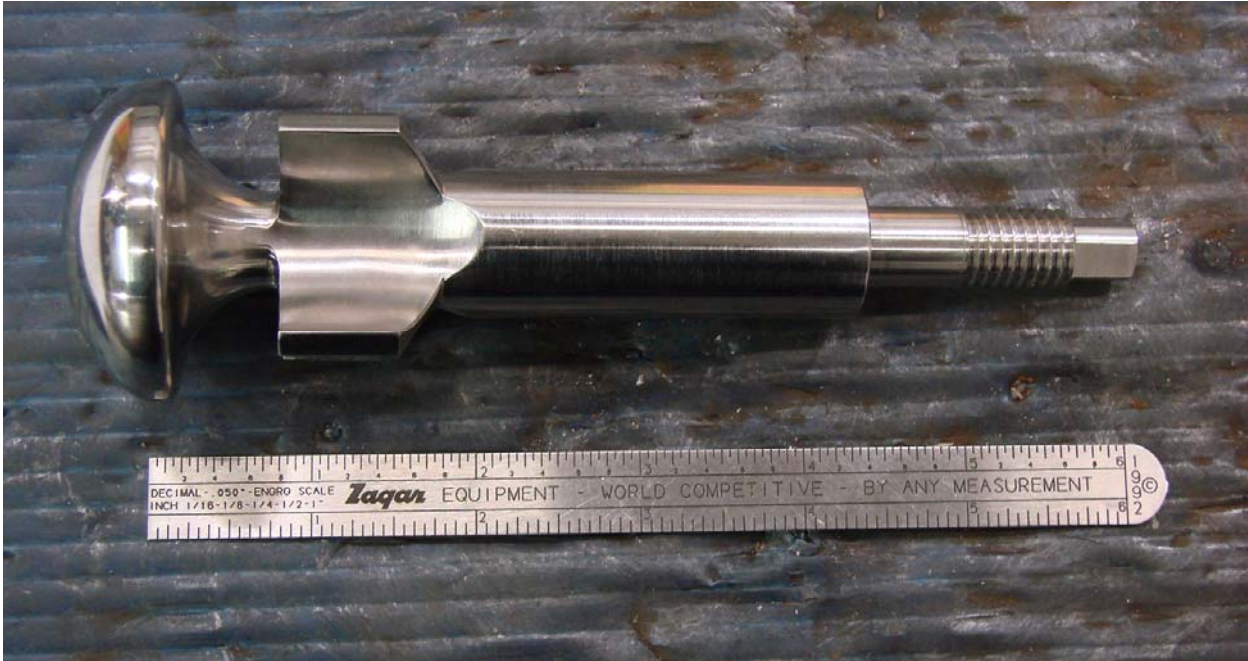
Figure B1: Pressure regulator valve of 316 stainless steel for operation in a 316L body in steam at 350°F. New valve that was subjected to SAT-12 treatment (valve supplied by Spirax Sarco).
