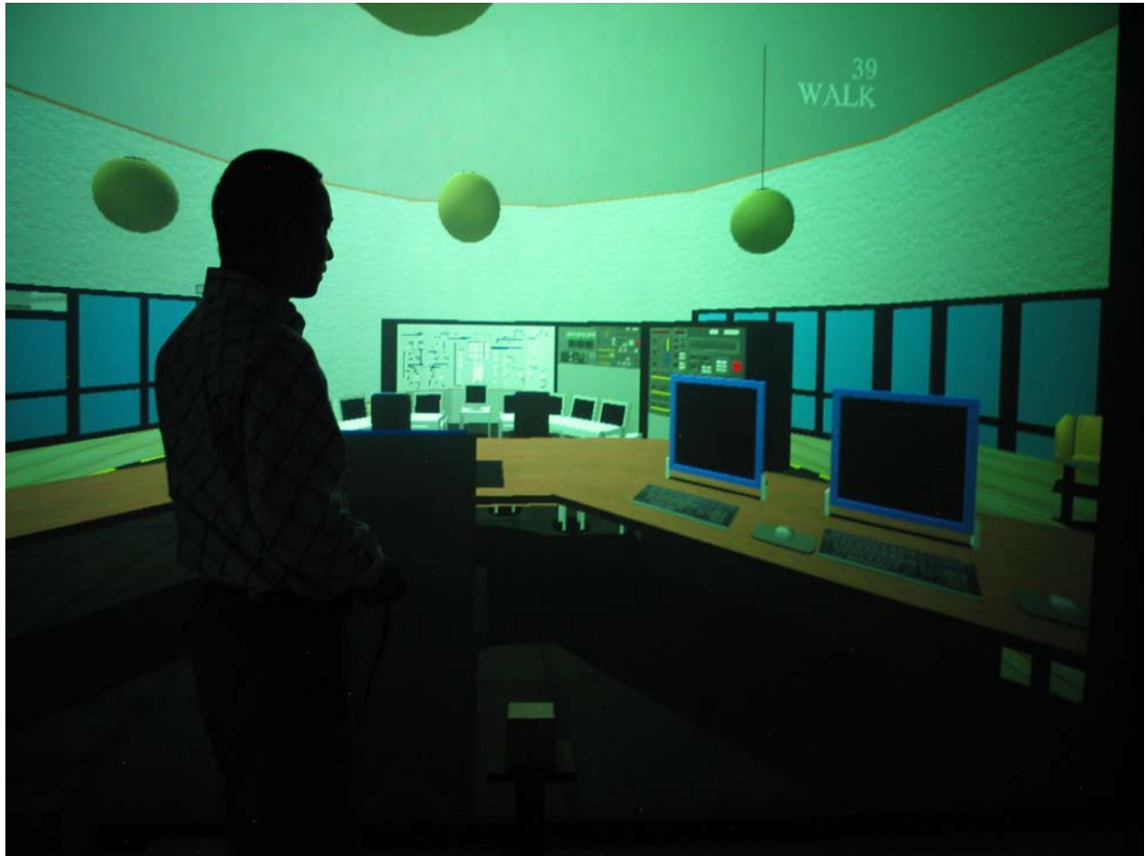
Figure B-2. A modern control room model being displayed—with an operator in the foreground (barely) shows that one can get a fairly realistic virtual experience in a VisBox.
