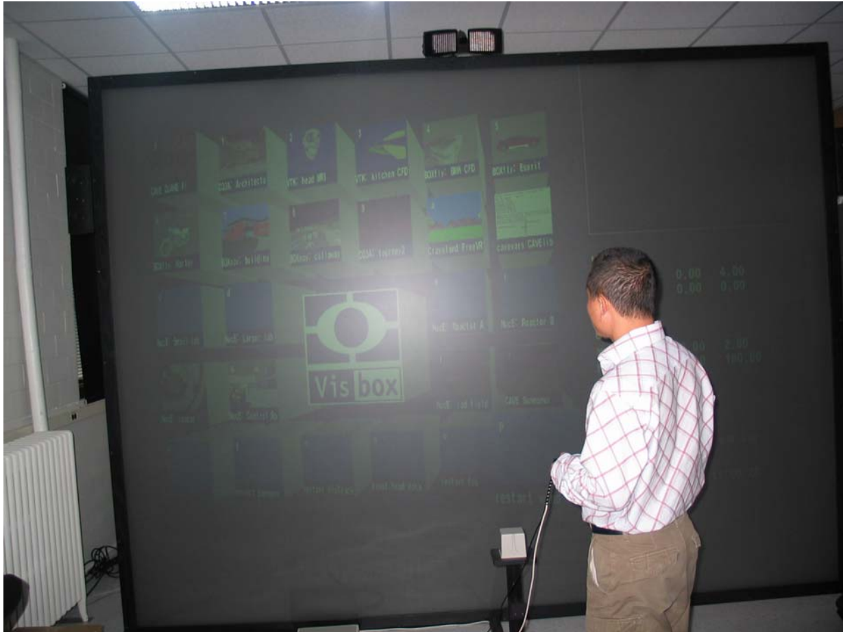
Figure B-1. A picture of the VisBox screen displaying the menu for several applications is shown. Any application can be selected using the game controller.
