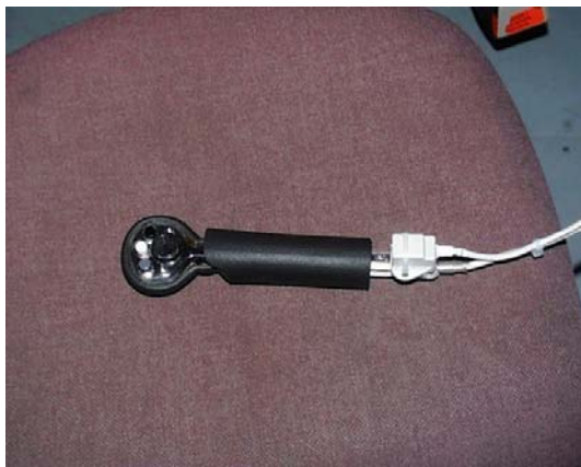
Fig. 4: The CAVE's input device, CAVE Wand, is an advanced 3D mouse/joystick with more degrees of freedom than a conventional device for a similar purpose.
