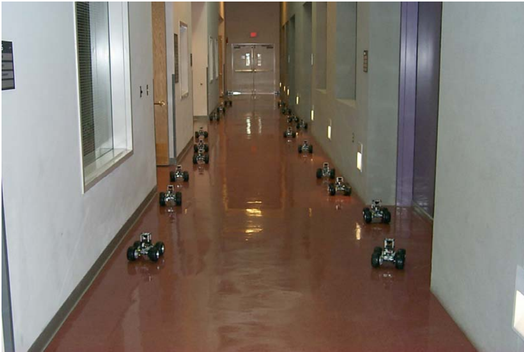
Figure 10. Surveillance task: starting in a single location, all 20 vehicles spread throughout the building while maintaining ultrasound and communication range to nearest neighbors.
