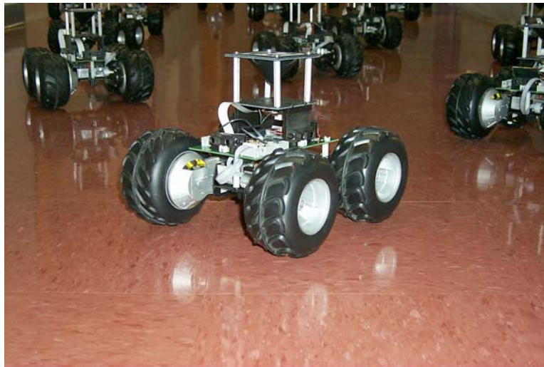
Figure 9. Robotic vehicle platform used in the tests.
