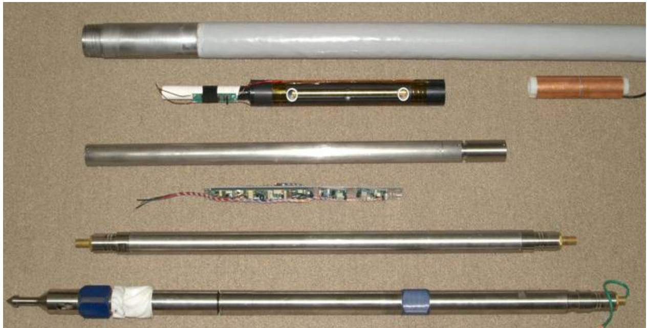
Figure 4-32. Major components of the initial drill string radar design. Shown top to bottom are the composite drill pipe, transmitter and receiver antennas, electronics enclosure, electronics chassis, downhole battery pack, and downhole turbine generator.
