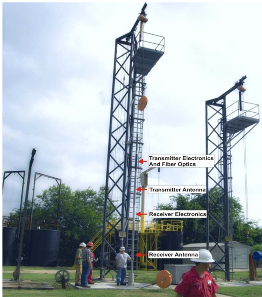
Figure 4-41. Prototype drill string radar tool prior to being lowered into the source borehole. The four major sections of the tool assembly are indicated.
