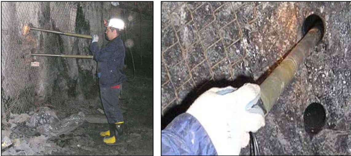
Figure 4-35. Proof-of-concept field testing of the drill string radar antennas in a coal mine.
